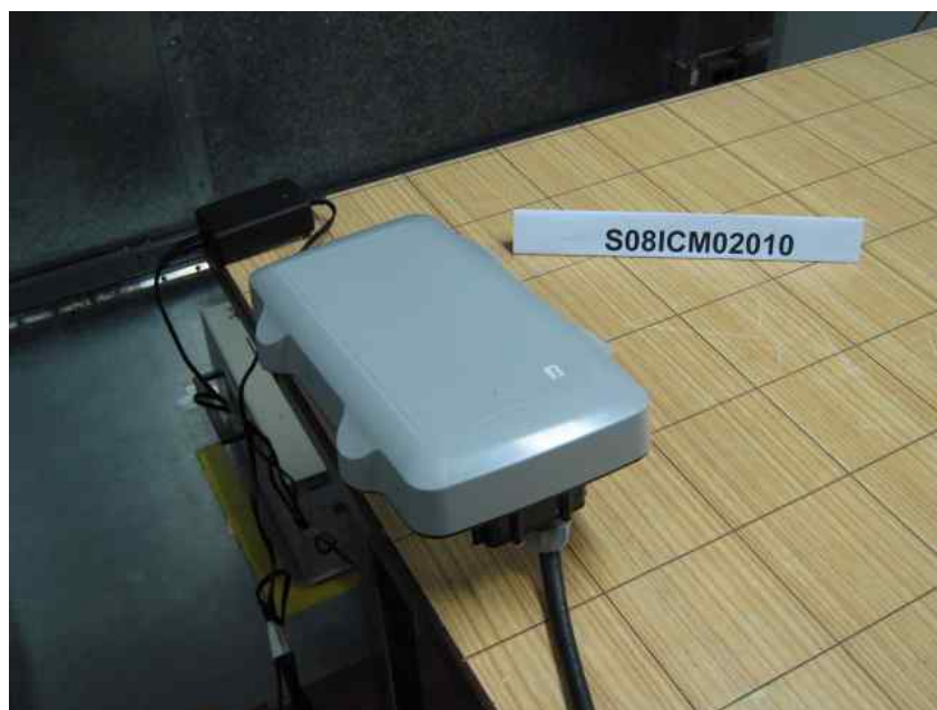
Conducted Emissions Test Setup (Rear View)
