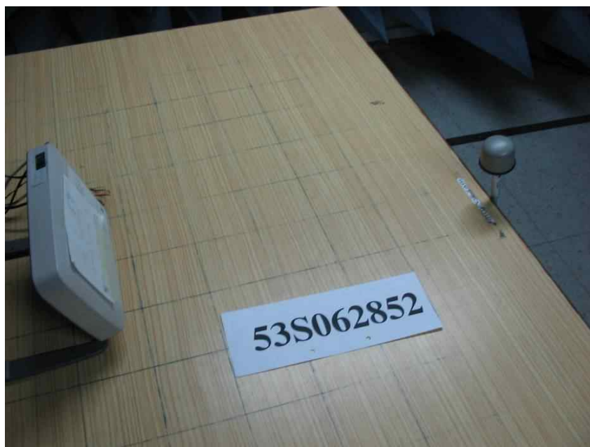
Maximum Permissible Exposure (MPE) Test Setup
