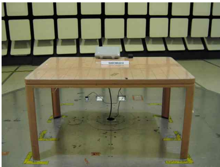
Radiated Emissions Test Setup (Front View)
