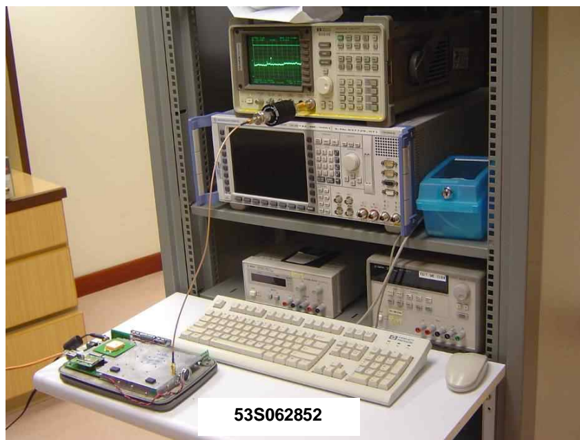
RF Output Power Test Setup
