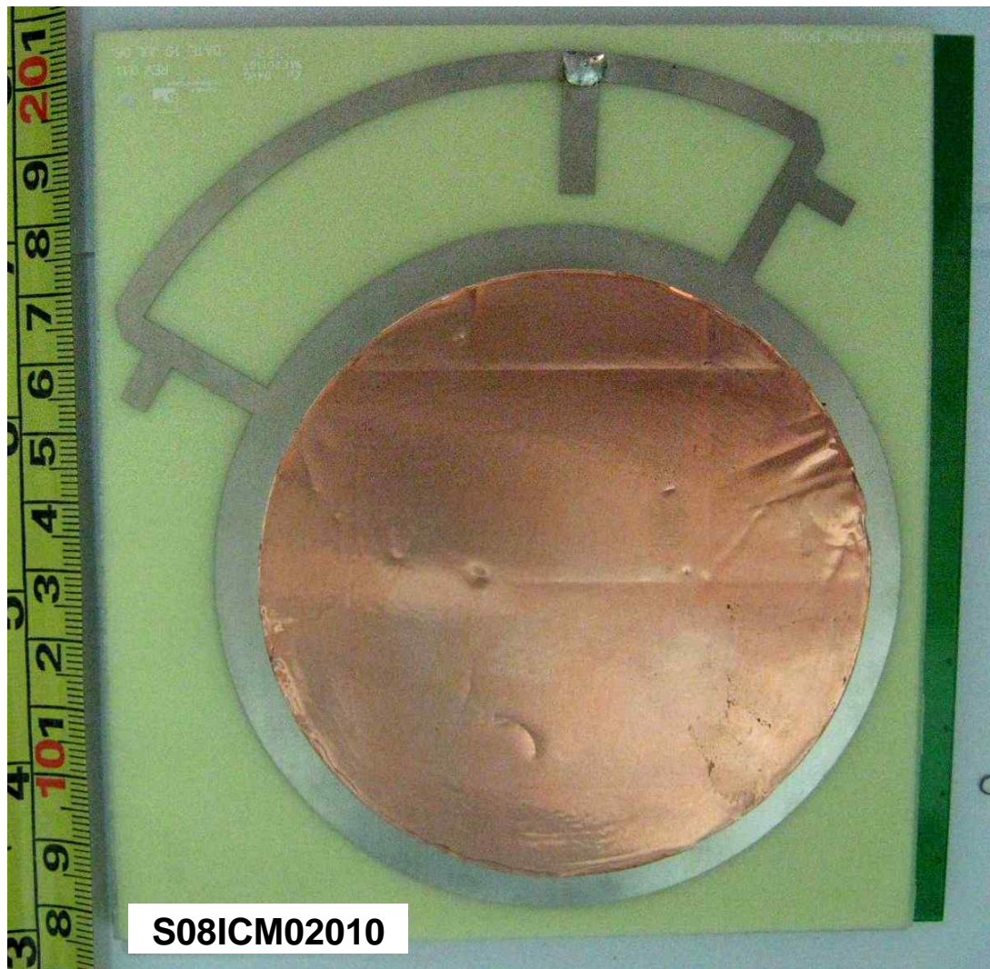
Lotus UT Antenna Board PCB Component Side
