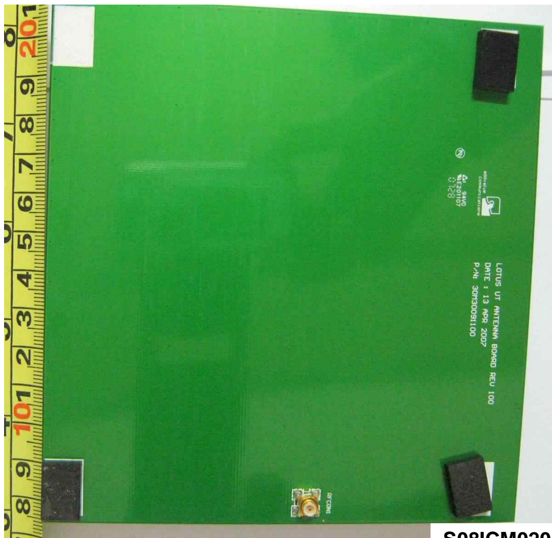
Lotus UT Antenna Board PCB Trace Side
