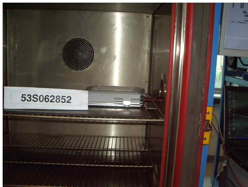
Frequency Stability (Voltage Variation) Test Setup
