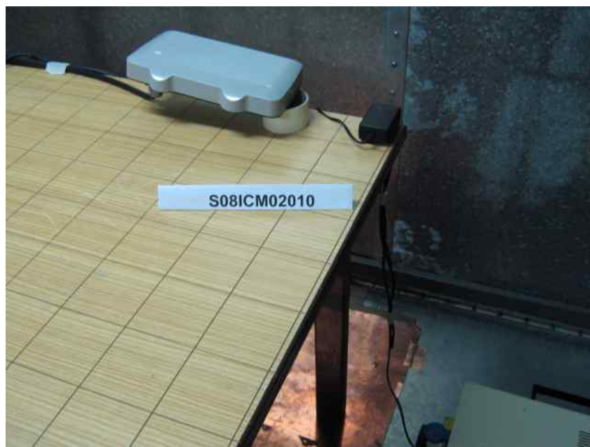
Conducted Emissions Test Setup (Front View)
