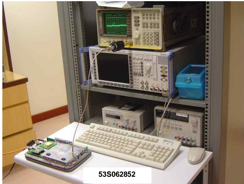
Unwanted Emissions at Antenna Terminal Test Setup
