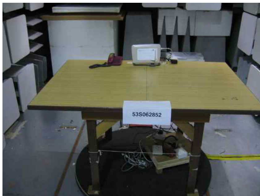
Radiated Spurious Emissions Test Setup (Front View)
