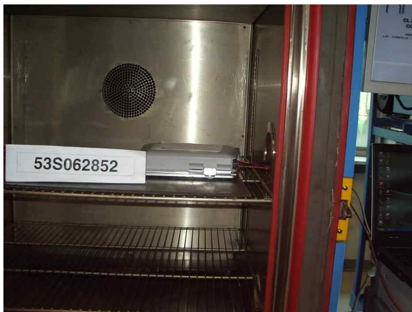
Frequency Stability (Temperature Variation) Test Setup
