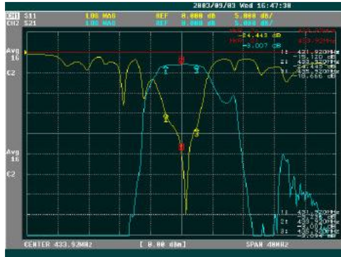
Figure 46: TX 433.92MHz IF filter response at 40MHz span.
