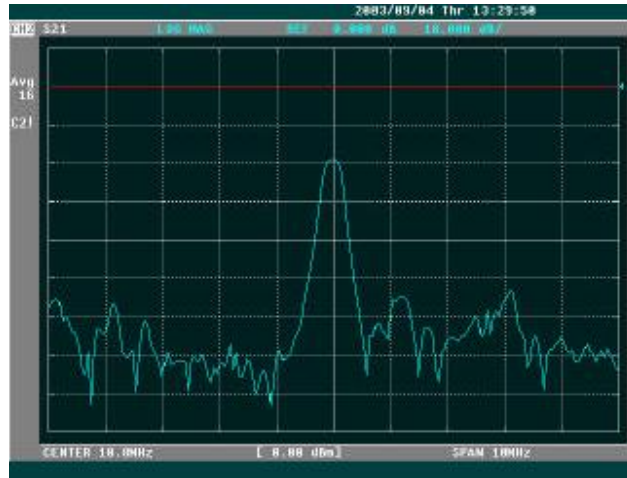
Figure 29: 2 nd RXIF (10.8MHz) filter response at 10MHz span.
