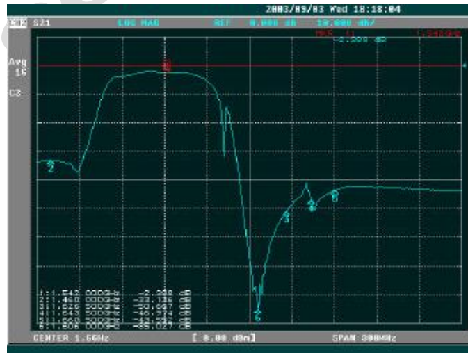
Figure 24: 1542MHz RF filter response indicating rejection to TX signal.
