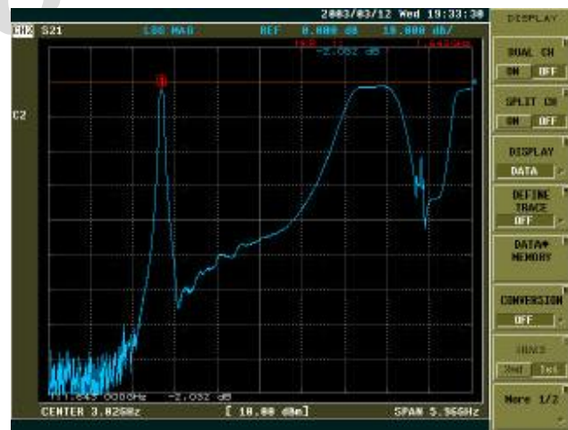
Figure 45: 1643 MHz filter response at 6000MHz span
