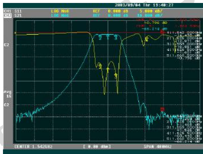
Figure 19: Duplexer – RX response at 400MHz span
