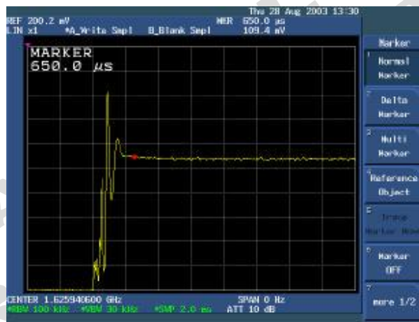
Figure 51: Switching time from 1660.5MHz to 1626.5MHz
