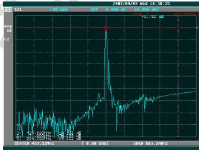
Figure 47: TX 433.92MHz IF filter response at 100MHz span.
