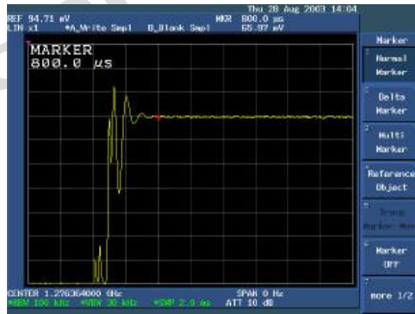
Figure 54: Switching time from 1310.4MHz to 1276.4MHz
