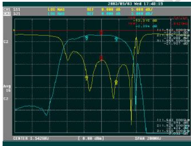
Figure 23: 1542MHz BPF response at span 200MHz
