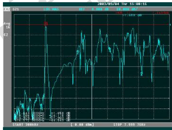
Figure 22: Duplexer – TX response at span 8000MHz
