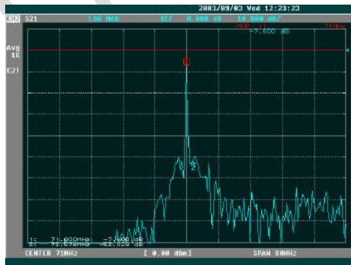
Figure 49: TX 71MHz IF filter response at 80MHz span.
