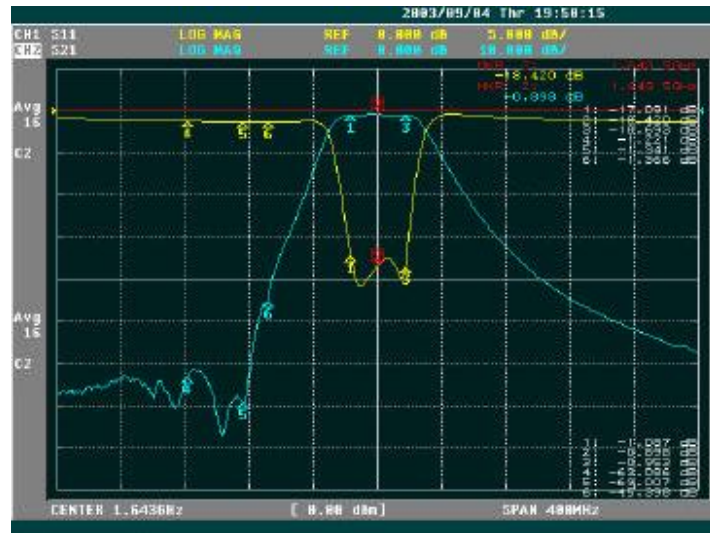
Figure 21: Duplexer – TX response at span 400MHz
