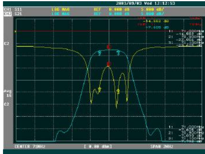
Figure 48: TX 71MHz IF filter response at 2MHz span.
