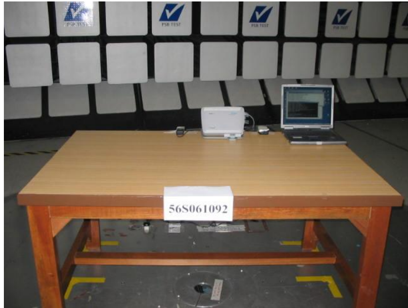
Radiated Emissions Test Setup (Front View)
