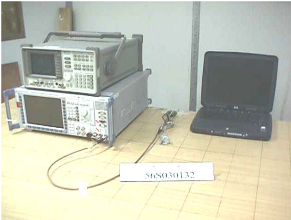
Number of Hopping Frequencies Measurement Test Setup
