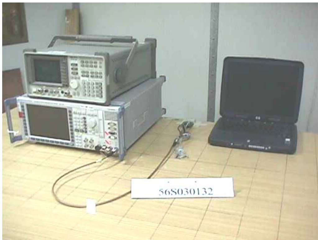
Effective Isotropic Radiated Power Measurement Test Setup
