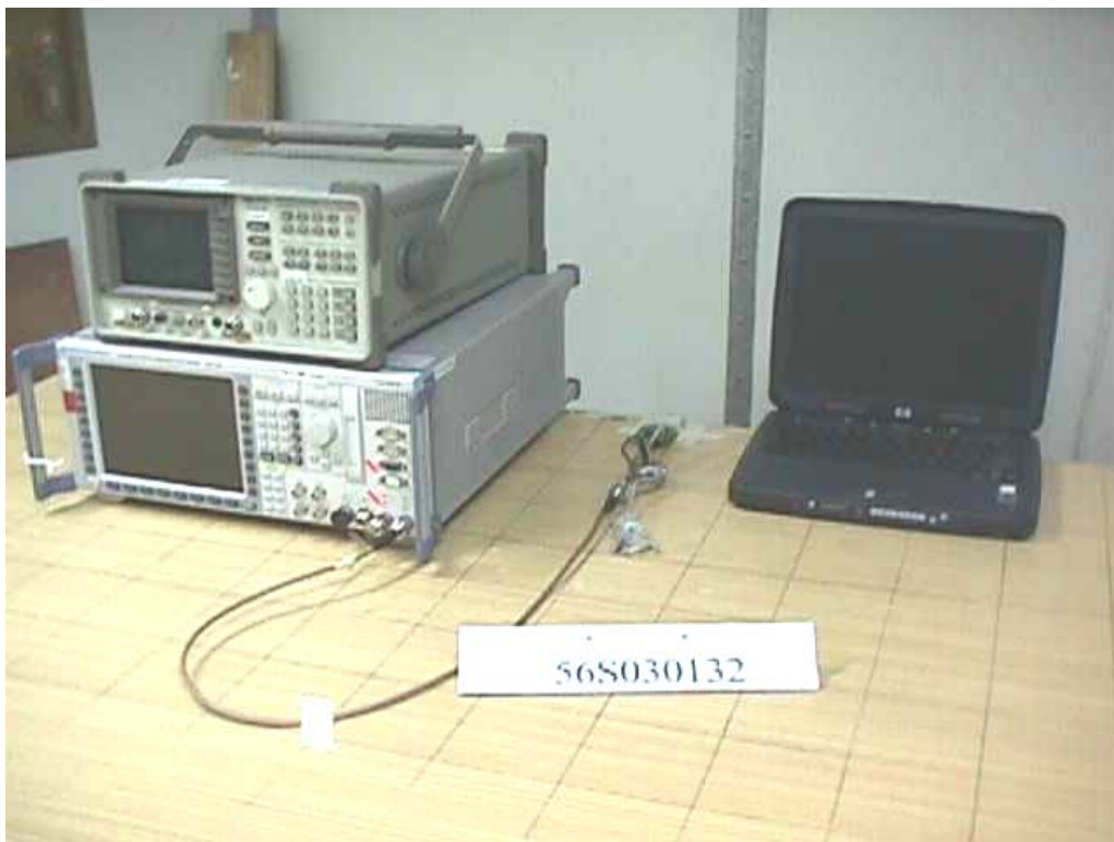
Maximum Peak Power Measurement Test Setup
