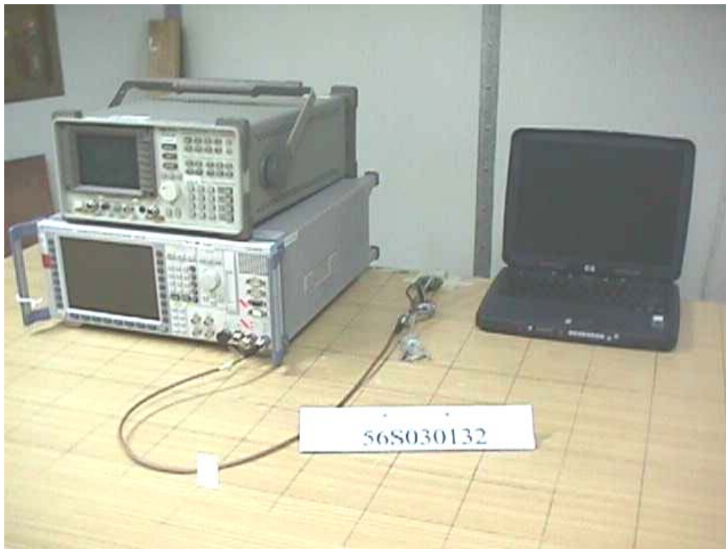
Peak Power Spectral Density Measurement Test Setup
