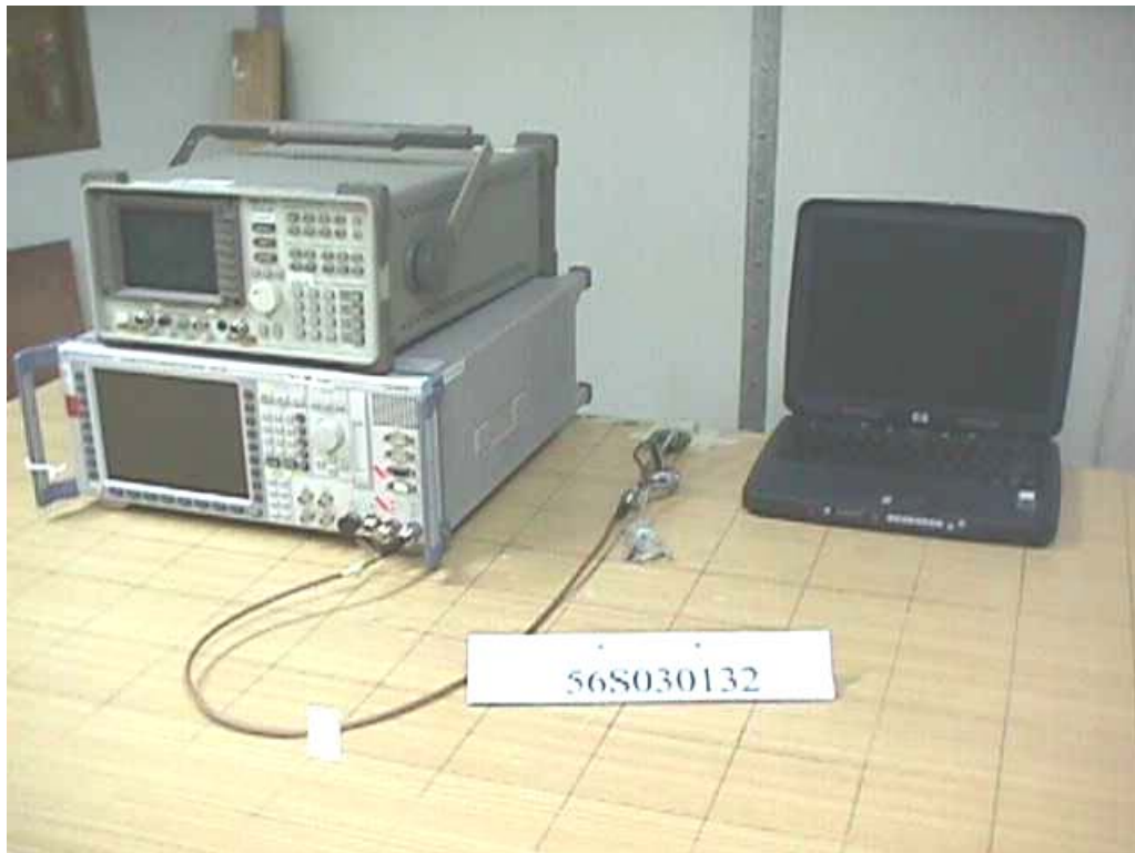
Average Frequency Dwell Time Measurement Test Setup
