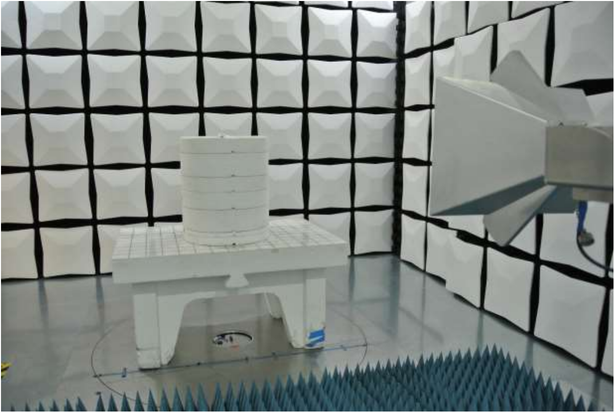
Figure 3: Test Setup for 1 GHz to 18 GHz (View 1)
