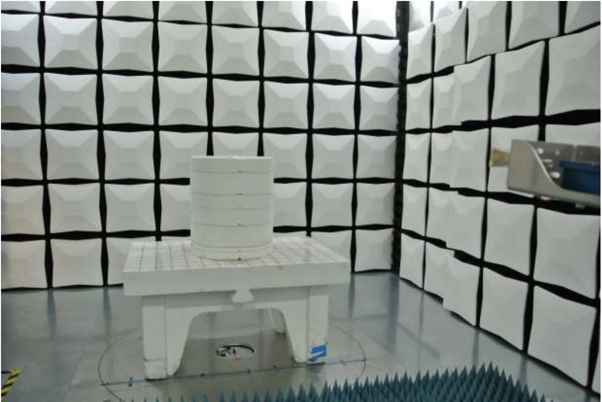
Figure 5: Test Setup for 18 GHz to 26GHz or 40 GHz (View 1)
