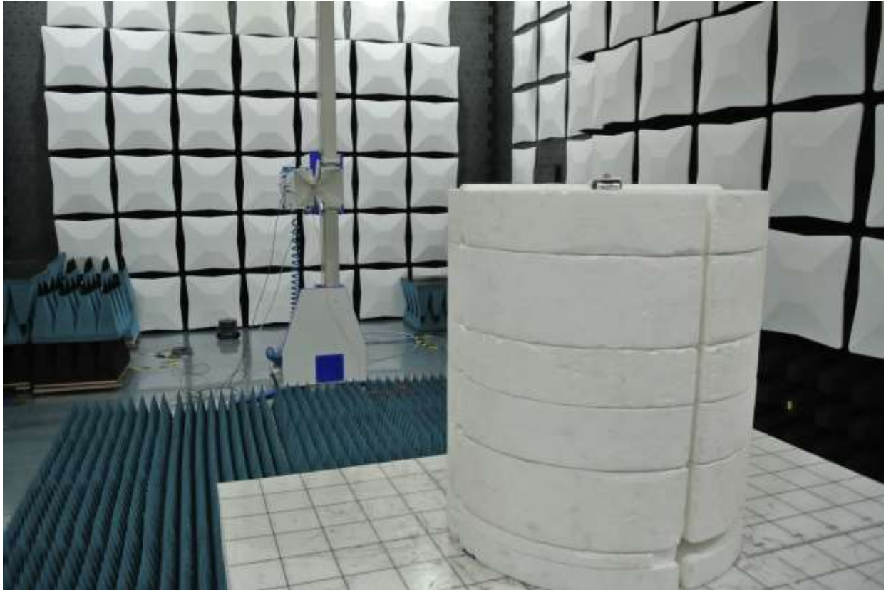
Figure 4: Test Setup for 1 GHz to 18 GHz (View 2)
