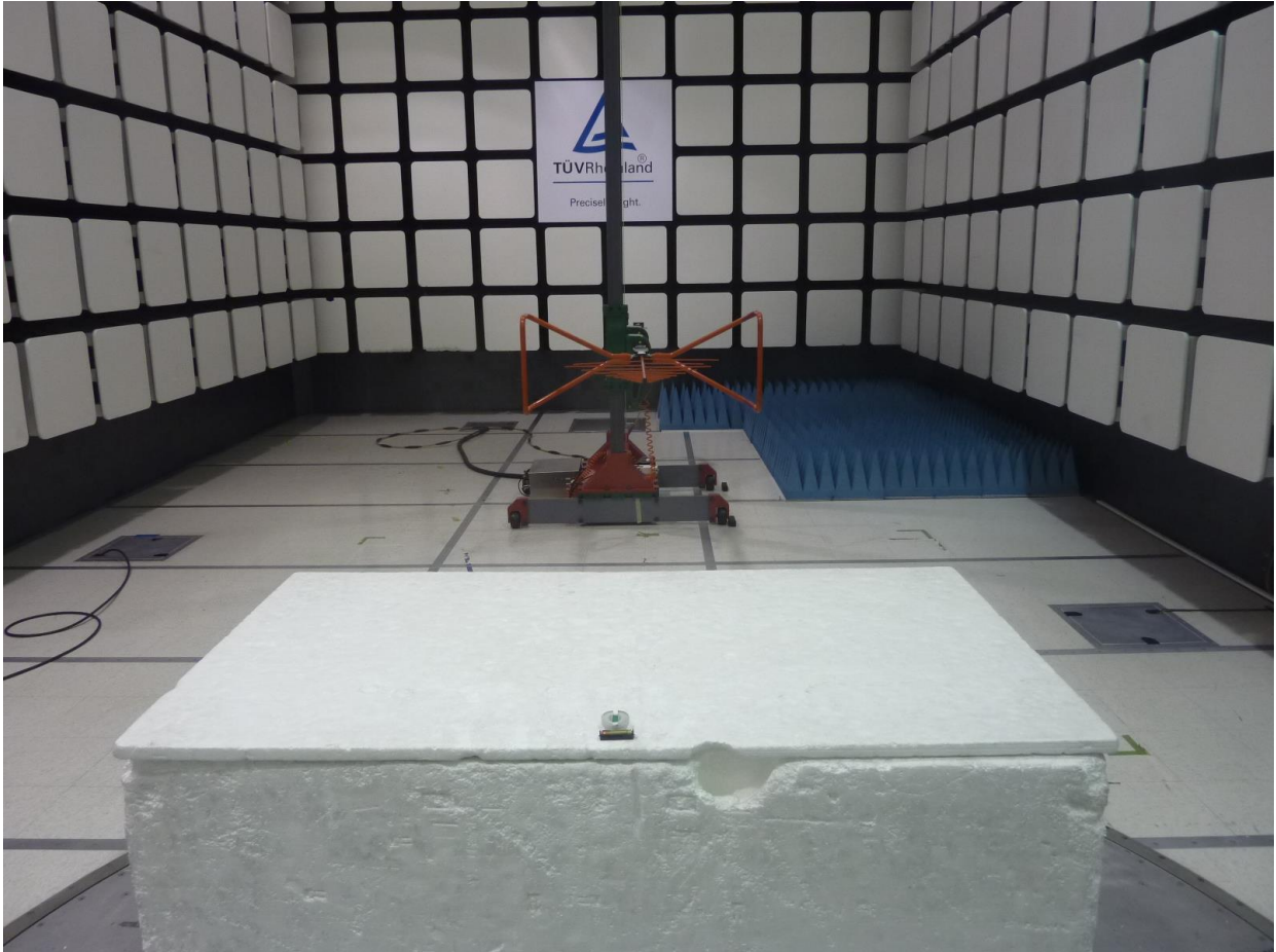
Figure 4: Test Setup for Radiated Emissions 30 MHz to 1000 MHz - Rear
