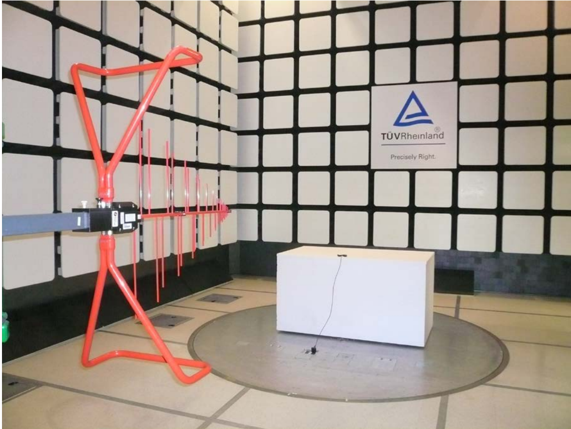
Figure 4: Test Setup for 30 MHz to 1000 GHz (Rear View)
