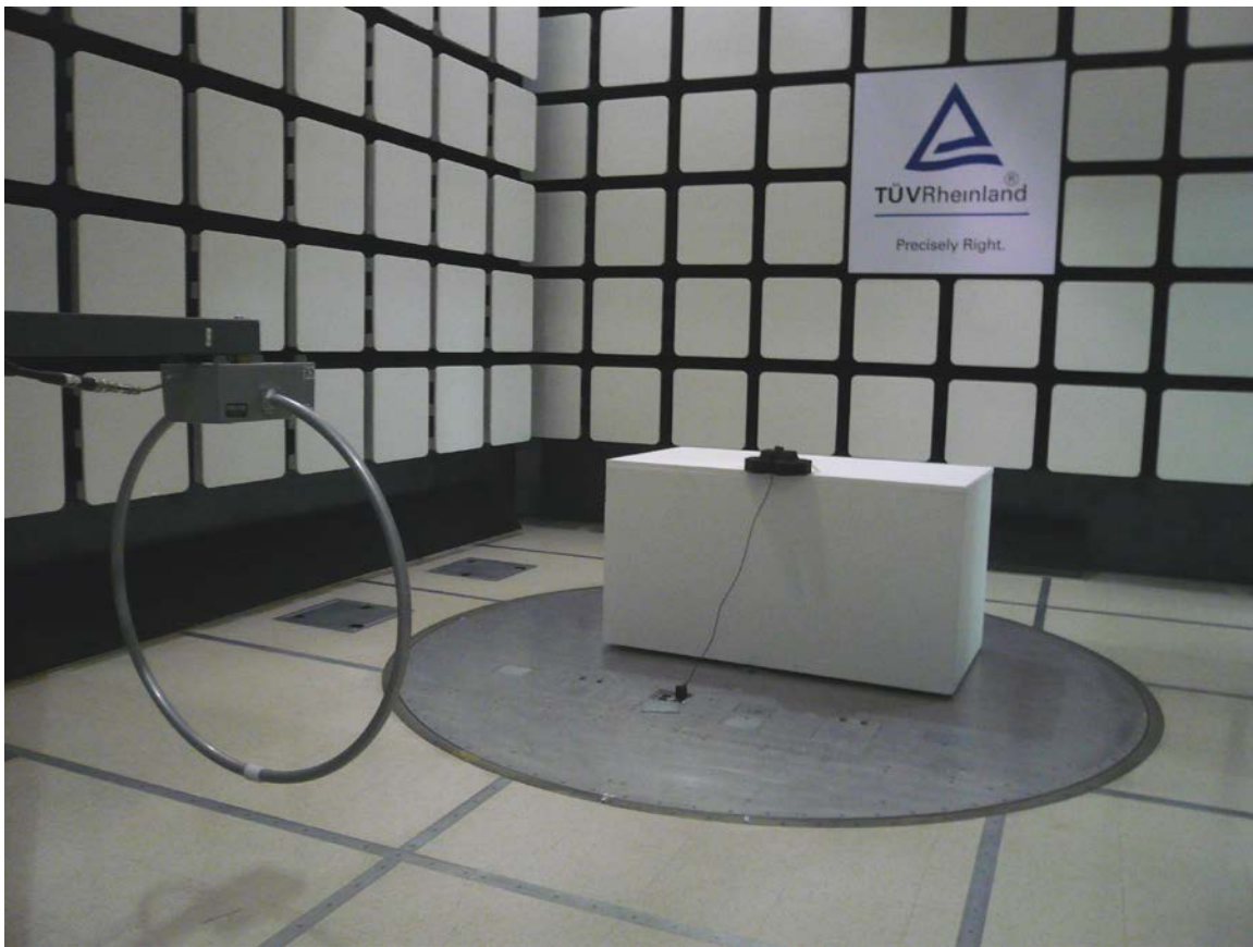
Figure 2: Test Setup for 9 kHz to 30MHz (Rear View) – Loop Facing EUT
