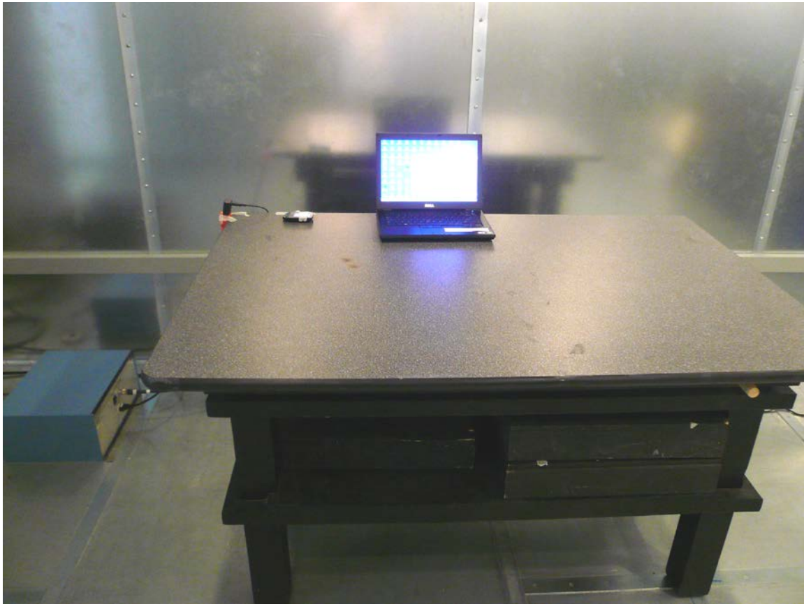
Figure 5: Test Setup for AC Conducted Emission (Front View)
