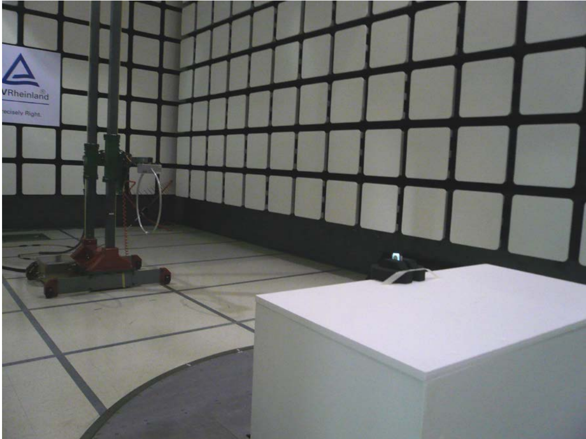
Figure 1: Test Setup for 9 kHz to 30MHz (Front View) – Loop Facing Away
