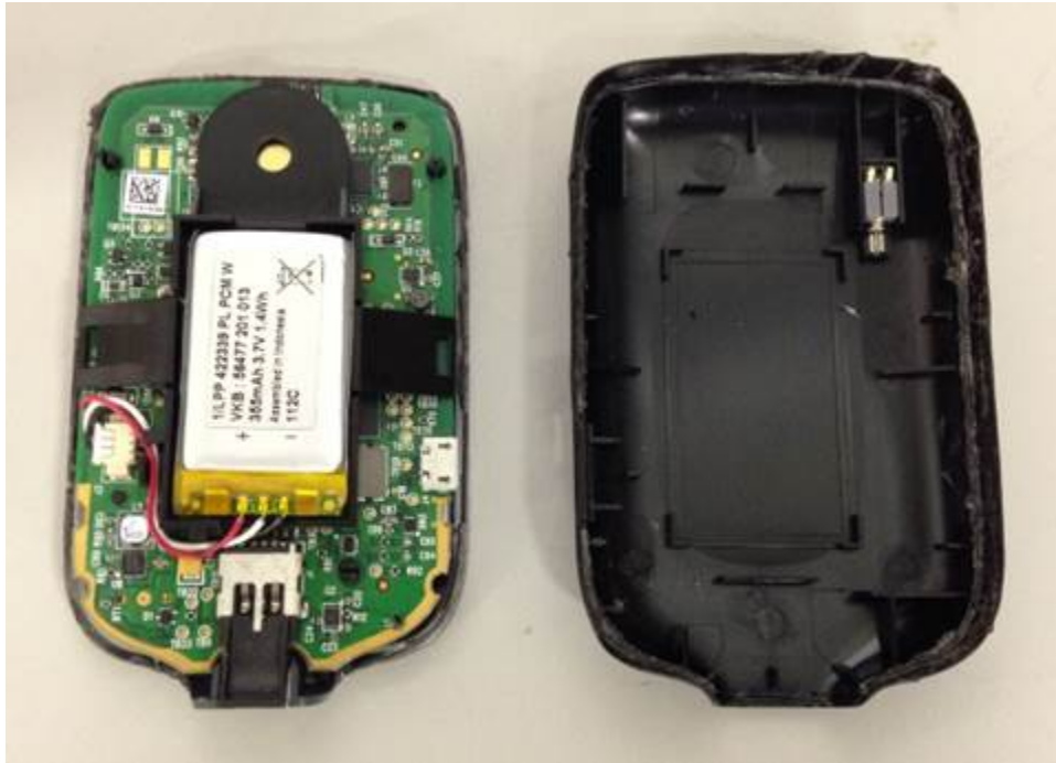
Photo 3 – Internal View of the Reader
