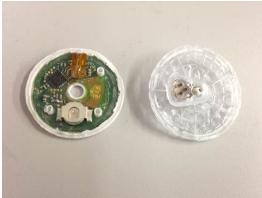
Photo 7 – Internal View of the Sensor
