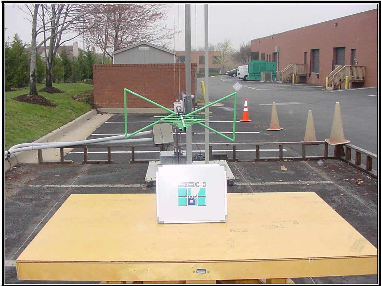
PHOTOGRAPH 2: RADIATED EMISSIONS (FRONT VIEW)
