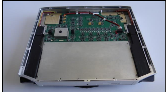
Internal Assembly without Transceiver assembly
