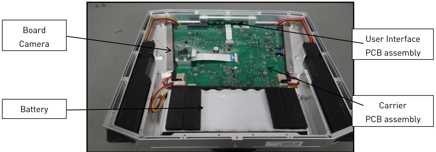
Internal Assembly without internal electronics shield
