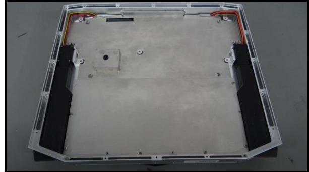
Internal Assembly without DC/IF PCB assembly and with internal electronics shield
