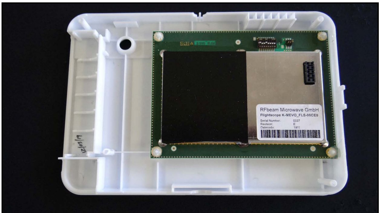
Front Enclosure with Microwave Board Assembly fitted and viewed from back side of Sensor.
