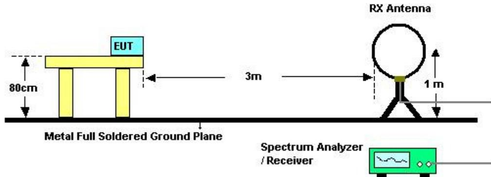
For Radiated Emissions: 30MHz~1GHz
