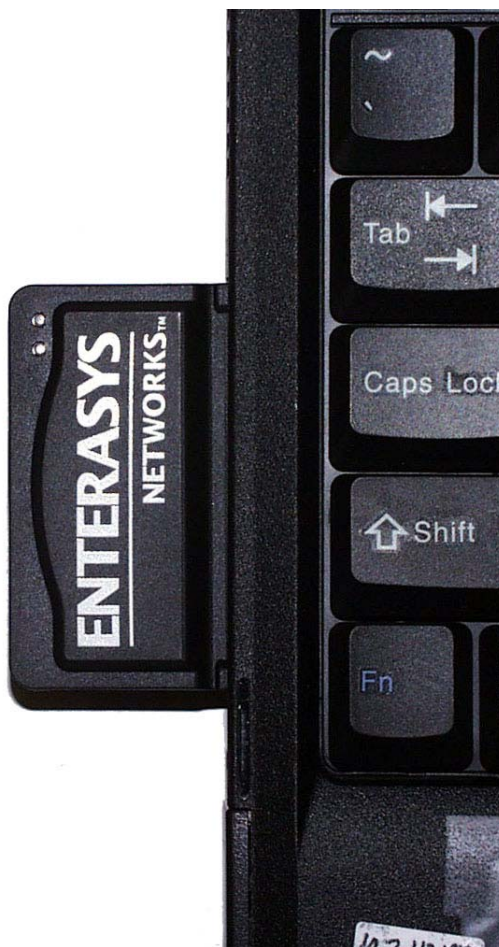
< LAN PC card installed in the host laptop >
