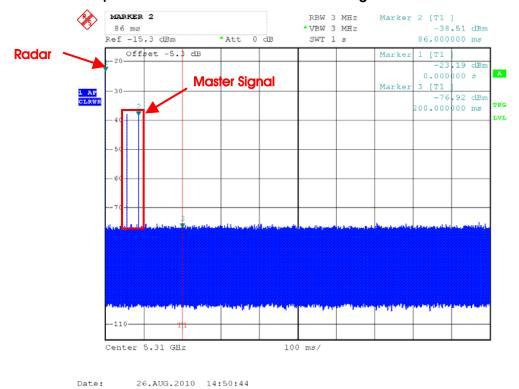
Radar #5 Channel Closing Transmission Time is comprised of 200 ms starting at the beginning of the Channel Move Time plus 30ms additional intermittent control signals. EUT have 0 control pulse.
