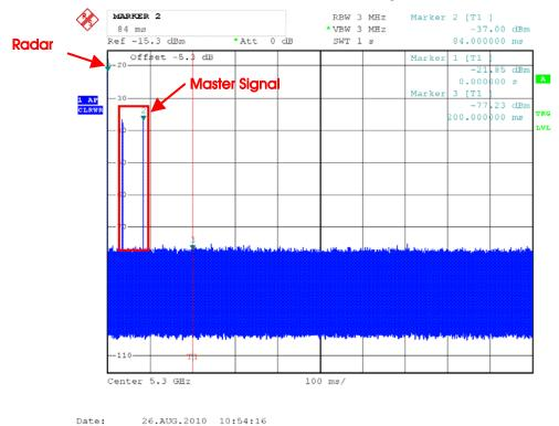
Radar #5 Channel Closing Transmission Time is comprised of 200 ms starting at the beginning of the Channel Move Time plus 30ms additional intermittent control signals. EUT have 0 control pulse.
