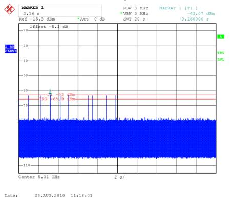
Radar #6 DFS detection threshold level and a single hop (9 pulses) on the Channel frequency within UNII detection bandwidth.
