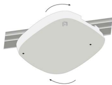
Figure 3 AP5010 access point ceiling install
