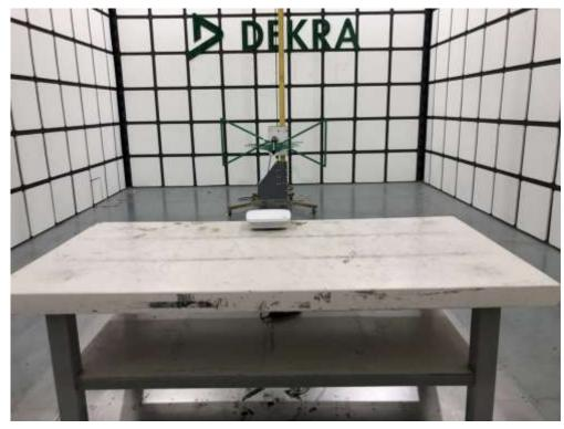
Description: Radiated Emission Test Setup for Below 1GHz(AP460C)
