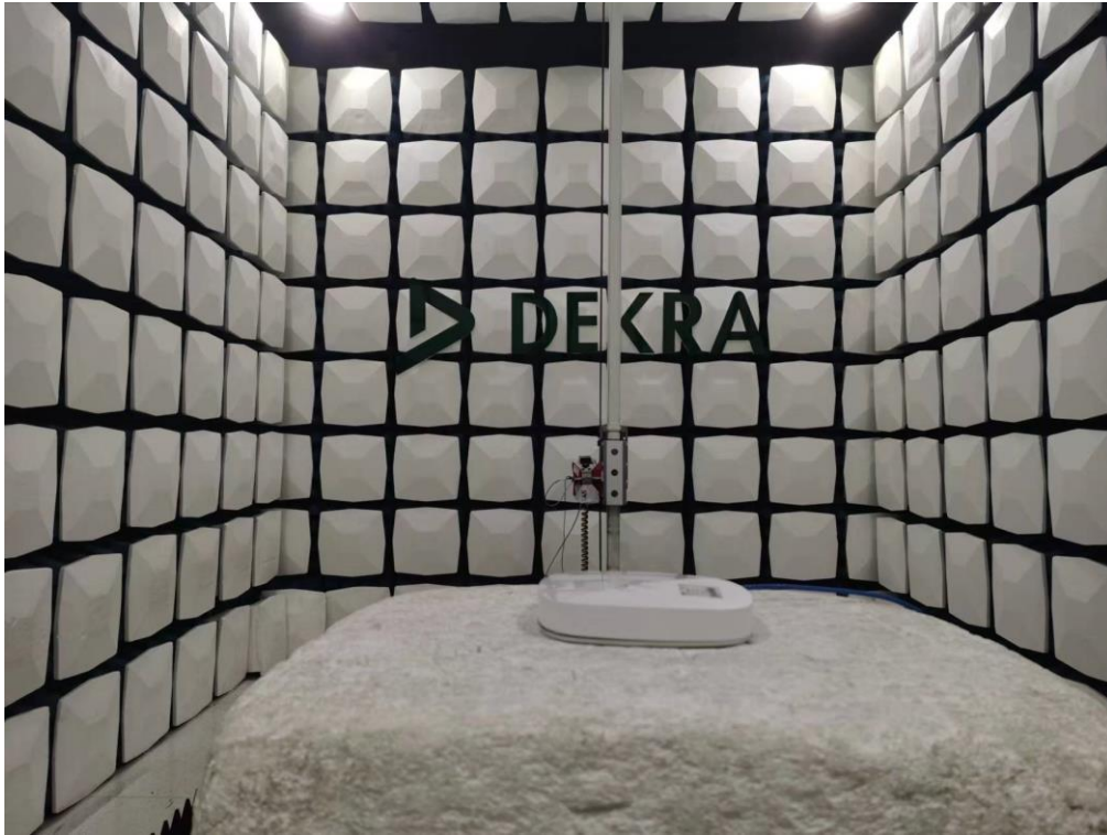
Description: Radiated Emission Test Setup for 1~18GHz
