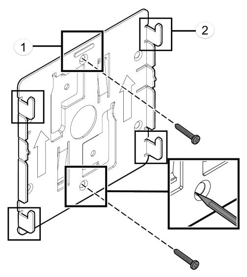
Figure 1: Main mounting bracket
