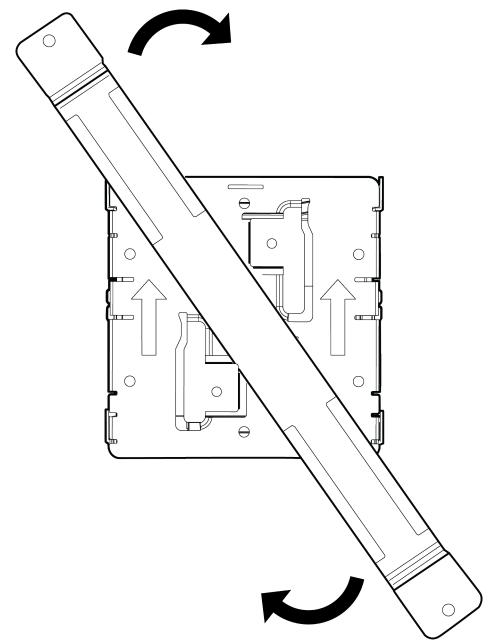
1 Keep the adapter to the center of the main mounting bracket, push and rotate it.
