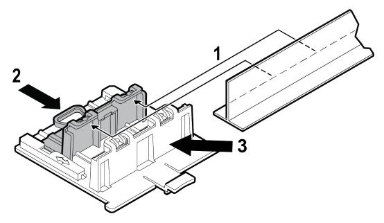
Figure 7: DCMTR01 bracket parts and T-bar
