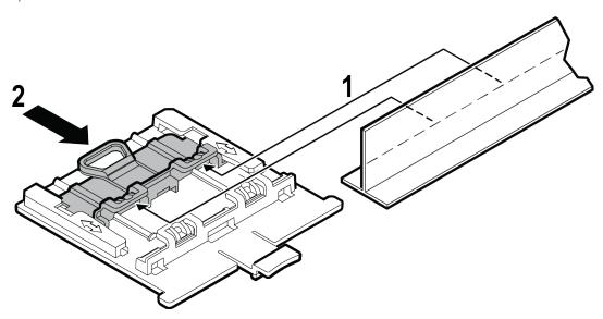
Figure 6: DCFLUSH bracket parts and T-bar
