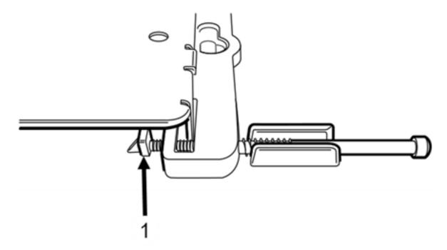
Figure 2: Security torx locking screw stop feature
