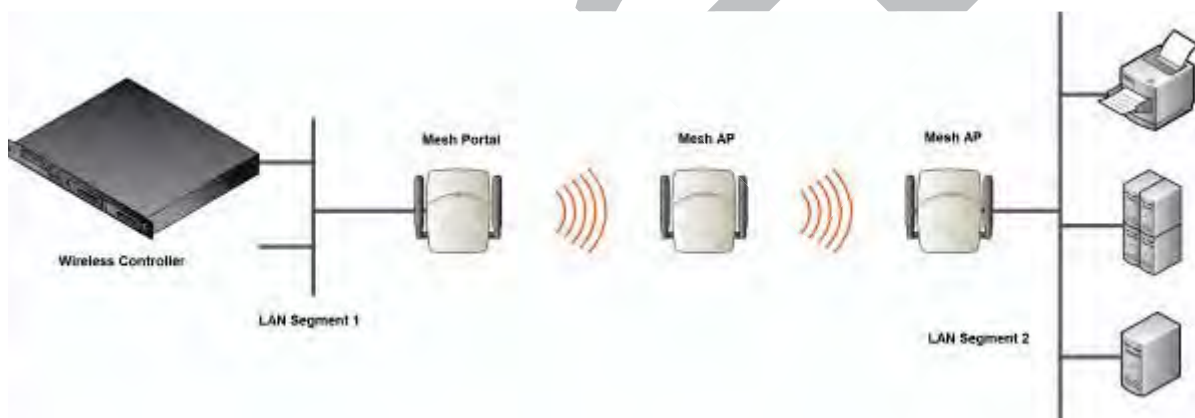
Figure 160: Wireless Bridge Configuration
