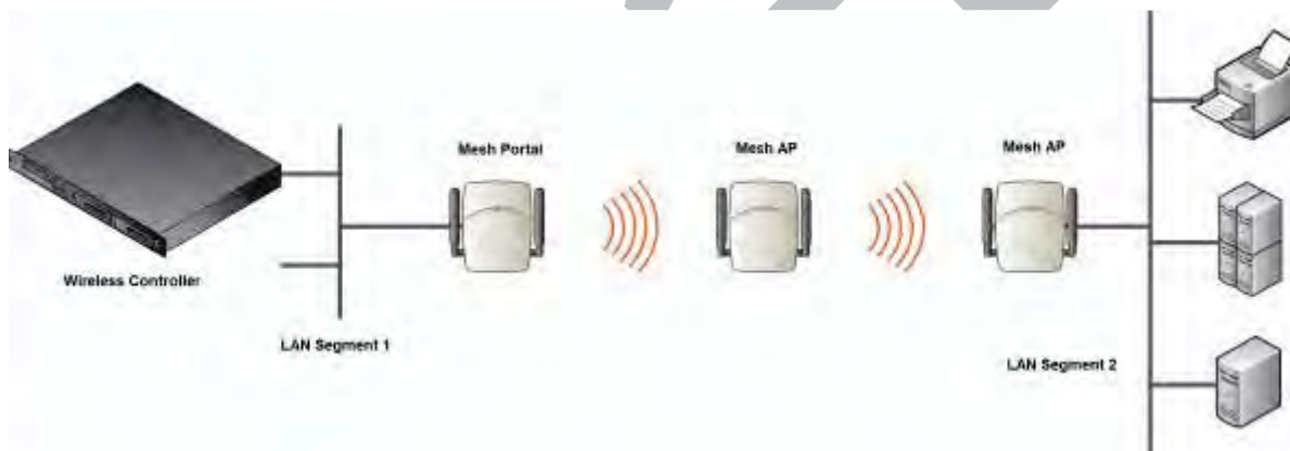
Figure 150: Wireless Bridge Configuration
