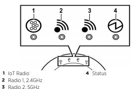
Green LEDs indicate 2G Wi-Fi Radio, Amber LEDs indicate 5.2G Wi-Fi Radio, and Blue LED indicates the IoT Radio. The Status LED is ON only during
