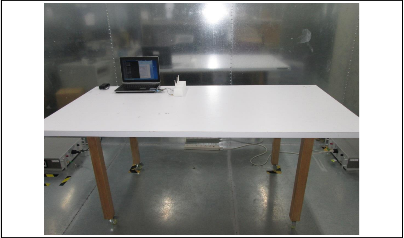
Conducted Emission Test _ Configuration 1
