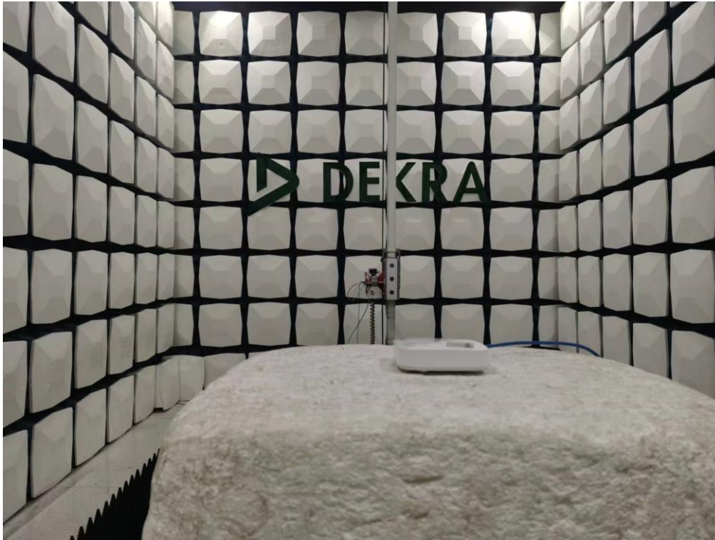
Description: Radiated Emission Test Setup for 1~18GHz
