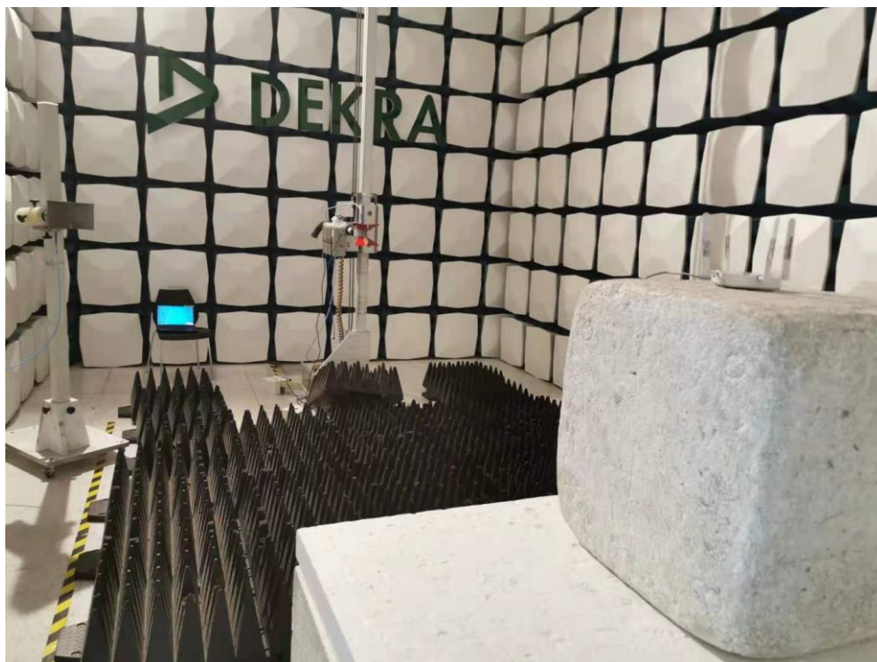
Description: DFS Test Setup(AP305CX)
