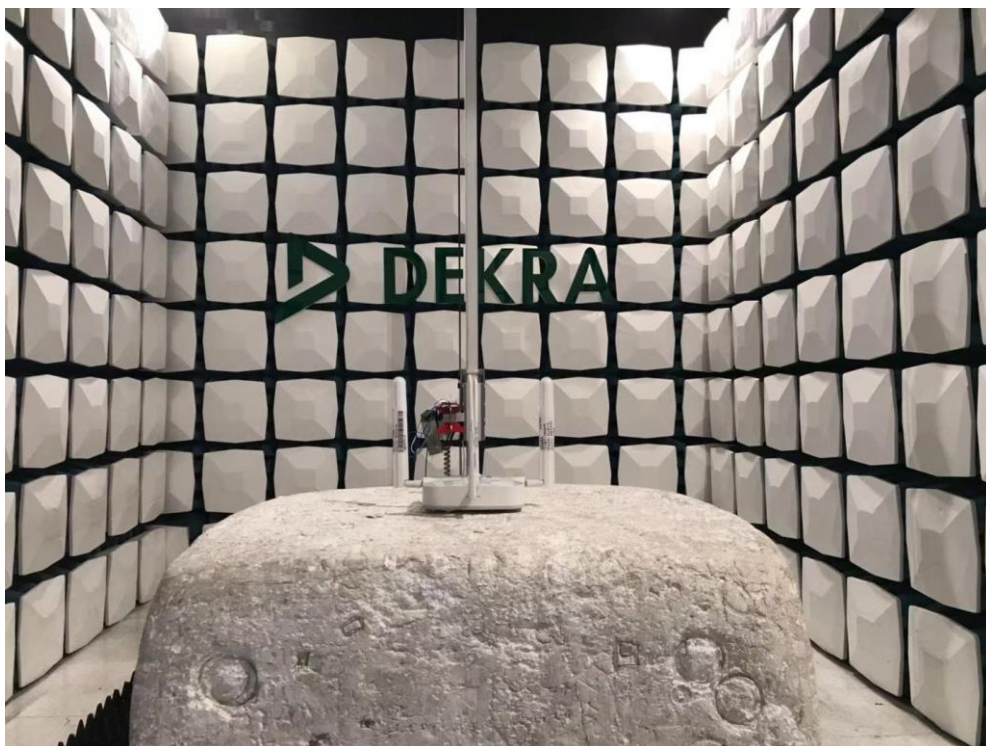
Description: Radiated Emission Test Setup for 1~18GHz(AP305CX)
