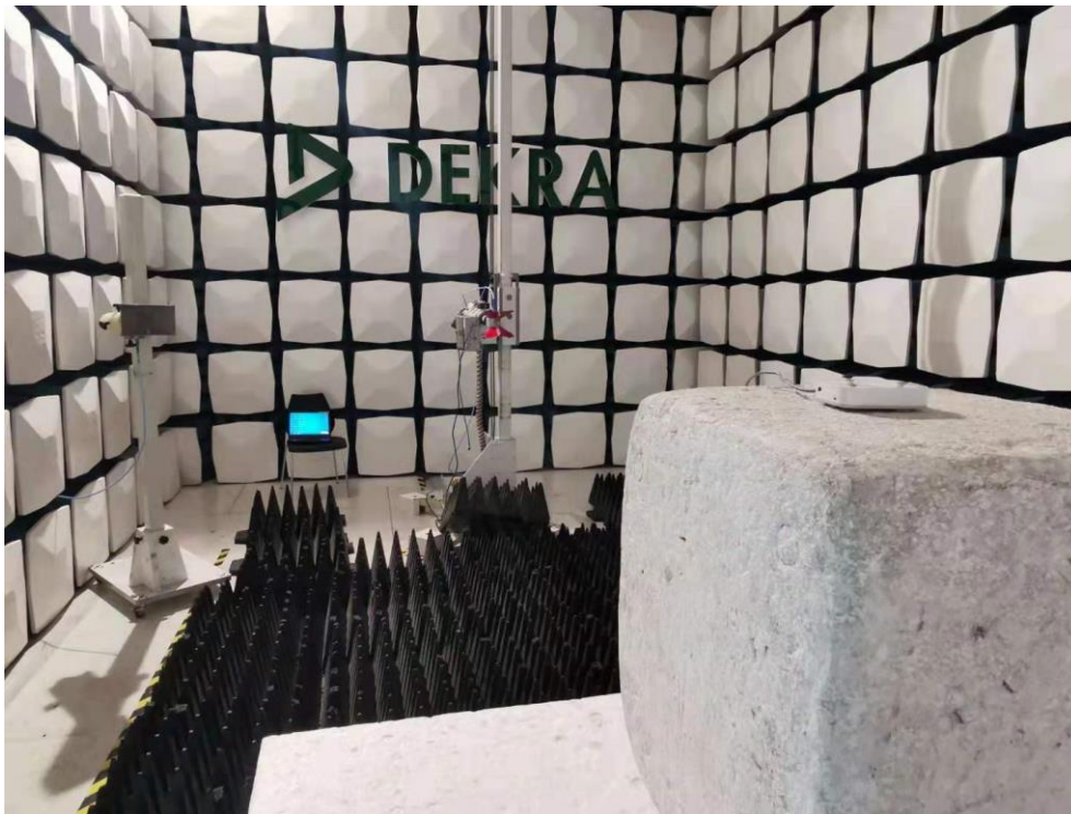
Description: DFS Test Setup(AP305C)
