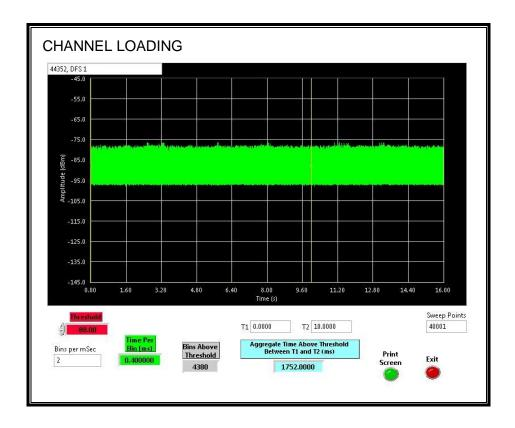
The level of traffic loading on the channel by the EUT is 17.52%
