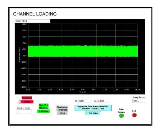
The level of traffic loading on the channel by the EUT is 17.496%
