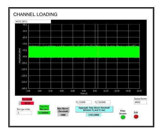
The level of traffic loading on the channel by the EUT is 17.632%
