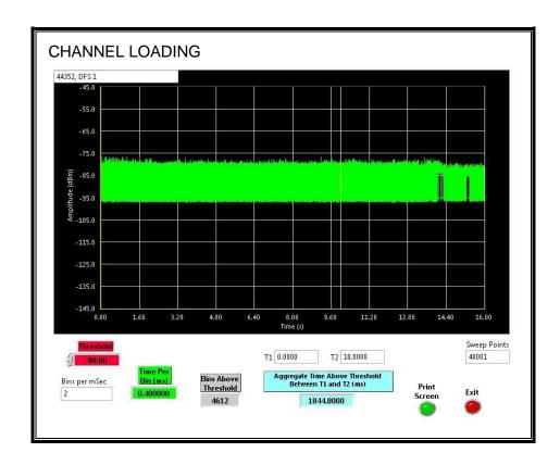
The level of traffic loading on the channel by the EUT is 18.448%
