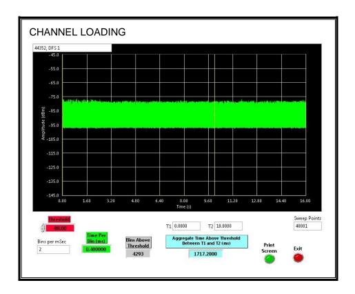
The level of traffic loading on the channel by the EUT is 17.172%
