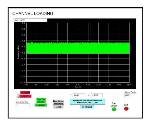
The level of traffic loading on the channel by the EUT is 17.992%
