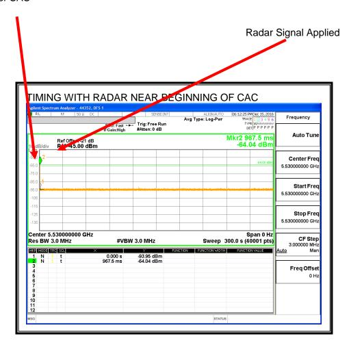
No EUT transmissions were observed after the radar signal.
