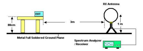
For Radiated Emissions: 30MHz~1GHz
