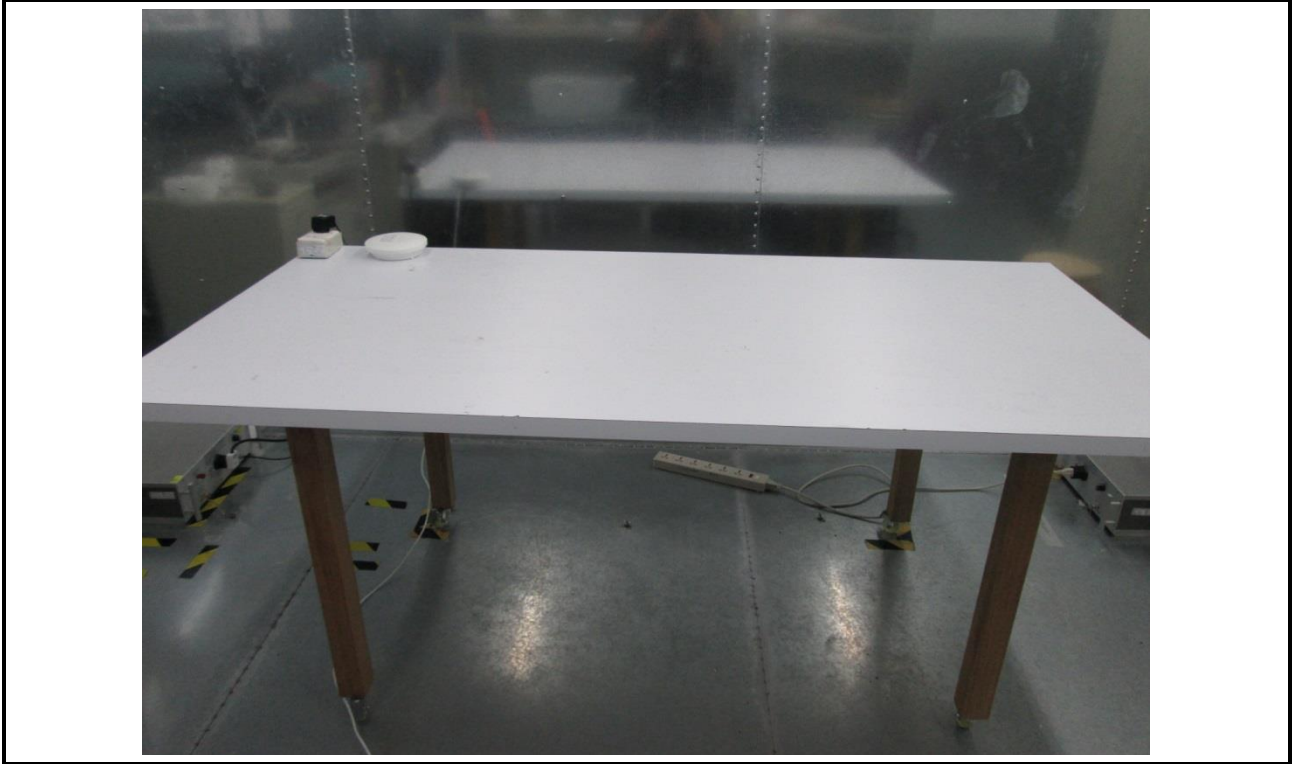
Conducted Emission Test (PIFA antenna, Adapter mode)
