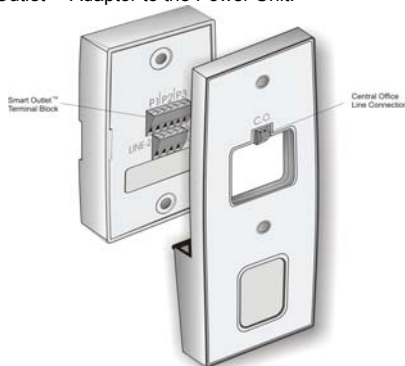
Figure 2.26: Rear Panel of Primary Smart Outlet™ Adaptor
