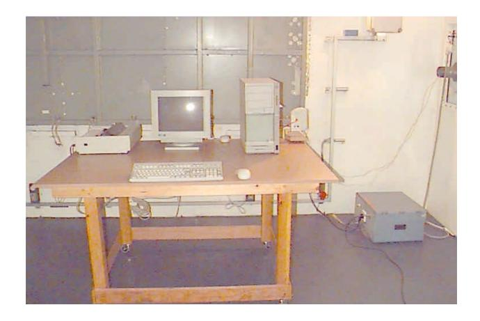
Photograph No.2 Radiated emissions measurement setup in the anechoic chamber with loop antenna
