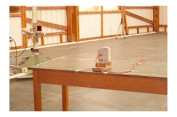
Photograph No.5 Radiated emissions measurement setup at the OATS, EUT view
