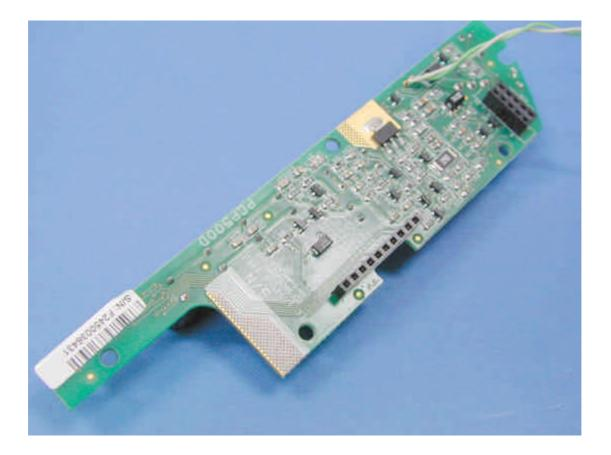
Photograph No.9 Wireless access point adapter PCB first side view
