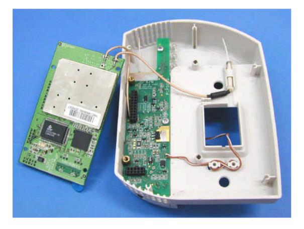
Photograph No.3 Wireless LAN Ethernet card front view
