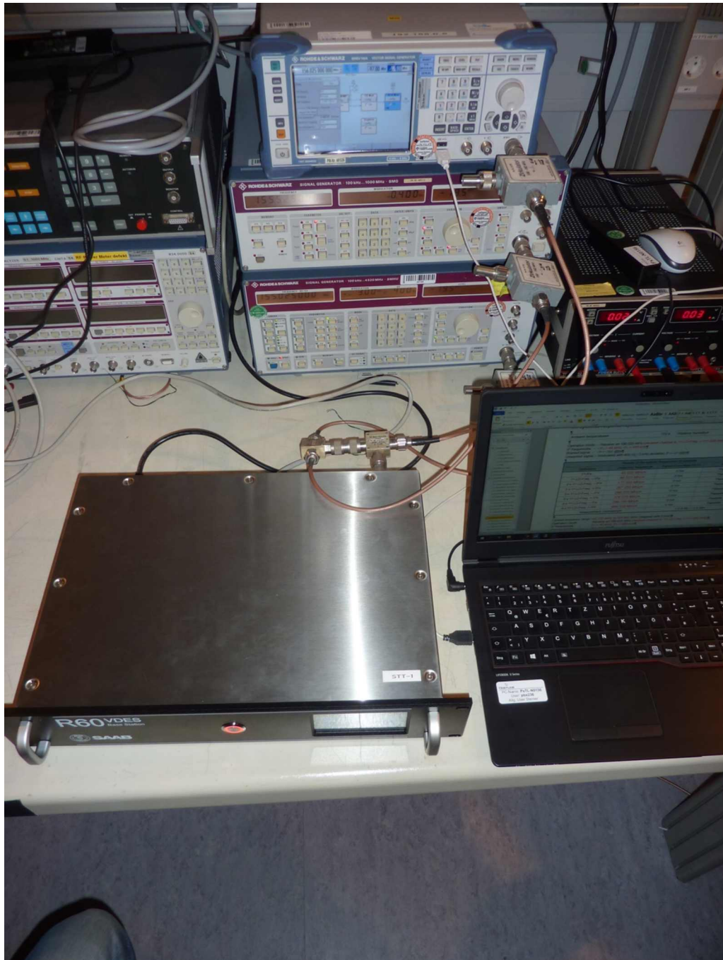
R60 VDES Base station, test set-up receiver tests
