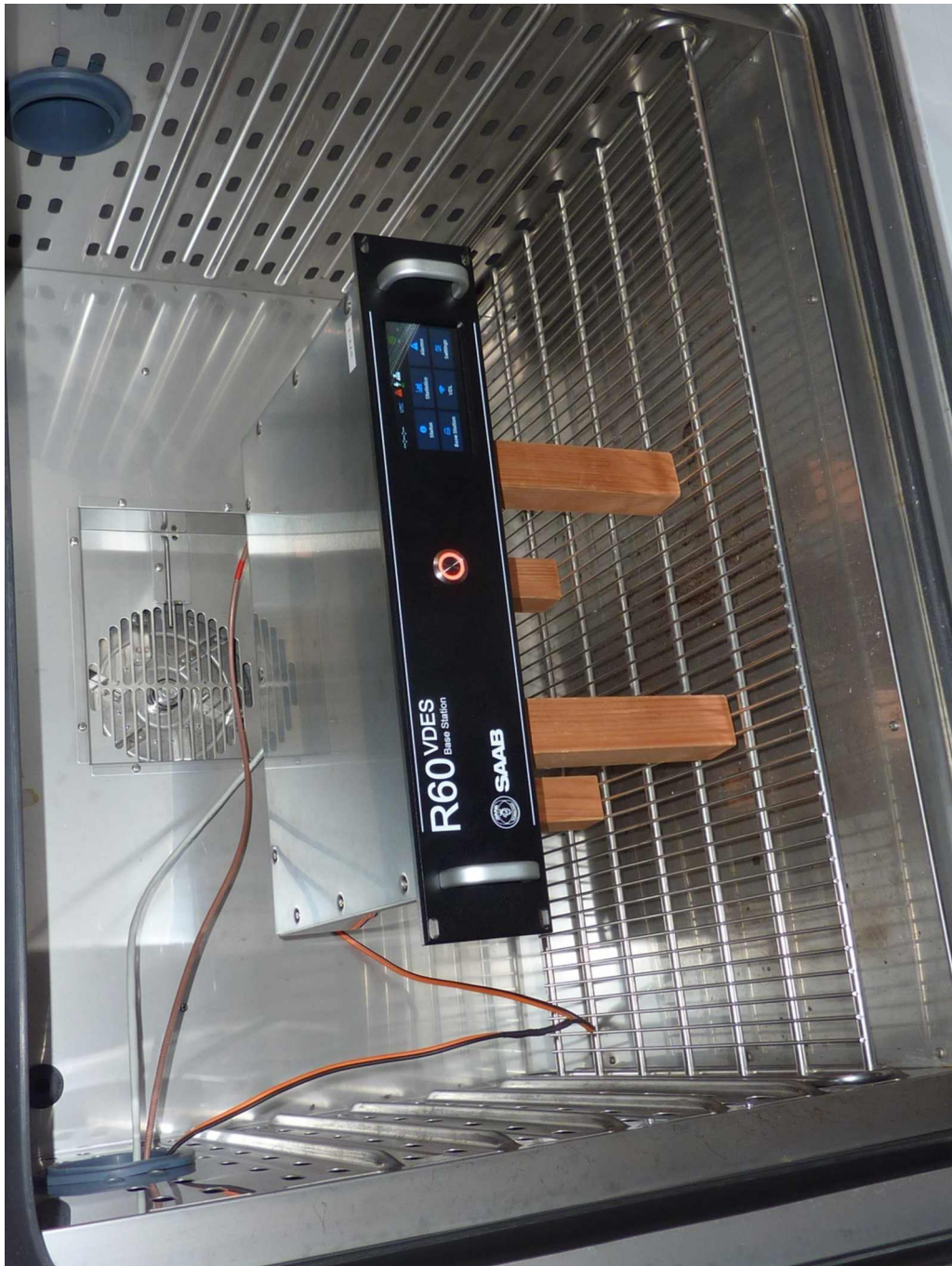
R60 VDES Base station, test set-up temperature chamber
