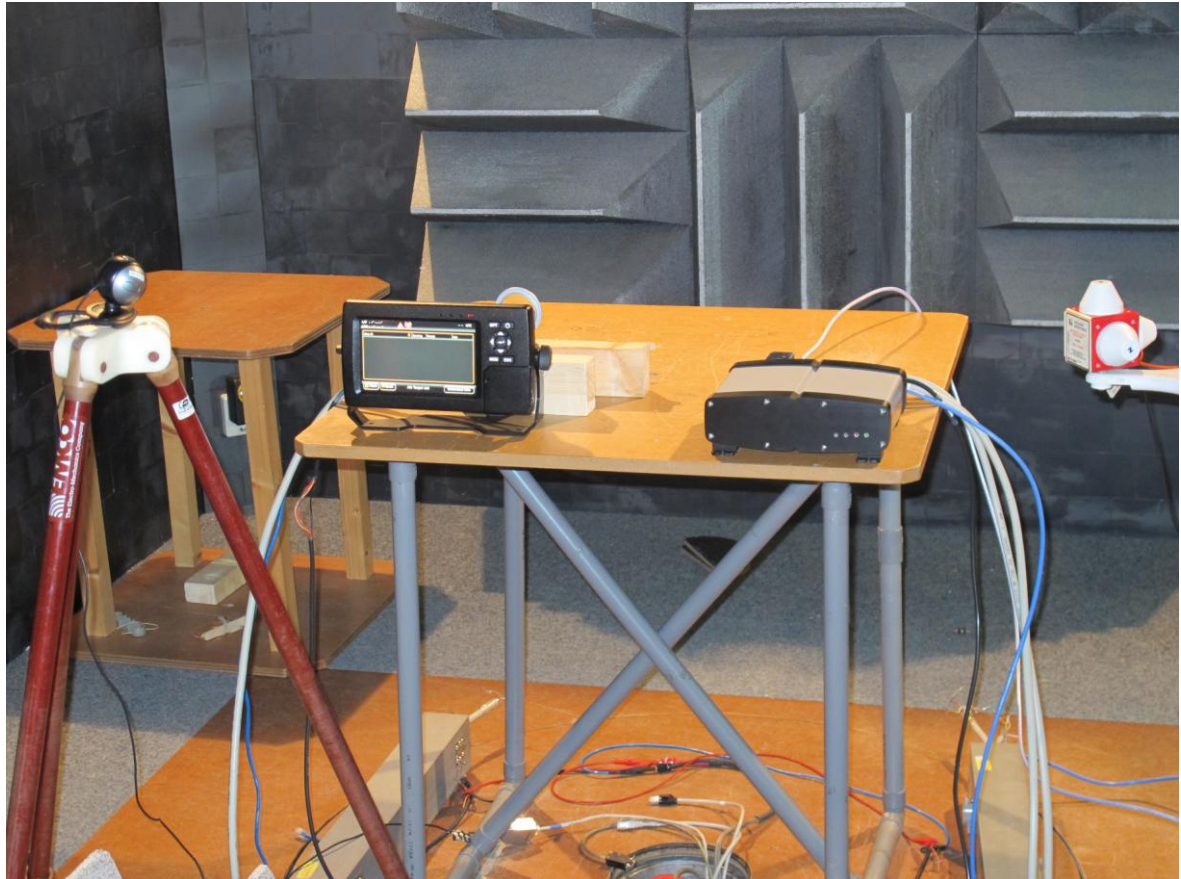
Photograph 8: radiated immunity test set up (0.08 – 1 GHz)
