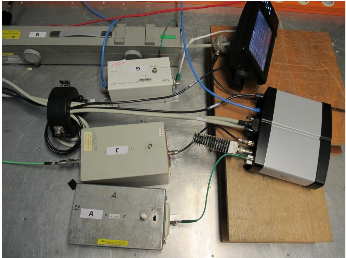
Photograph 9: Conducted immunity test set up (0.15 – 80 MHz)
