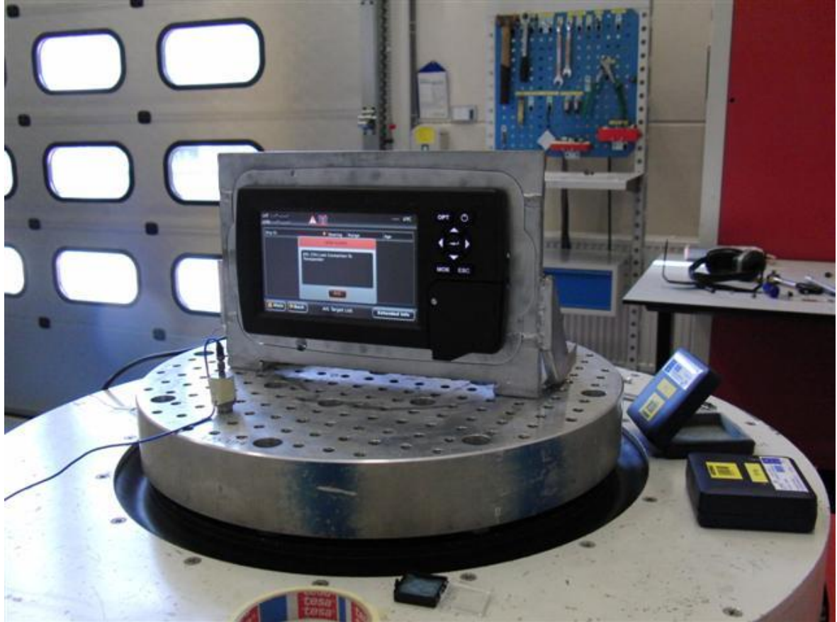
Photograph 13: Vibration test set up with R5 CDU in panel mounting frame (vertical direction)
