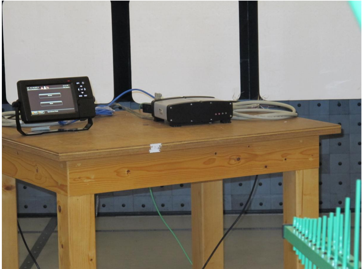
Photograph 7: radiated emissions test set up (0.03 – 1 GHz)
