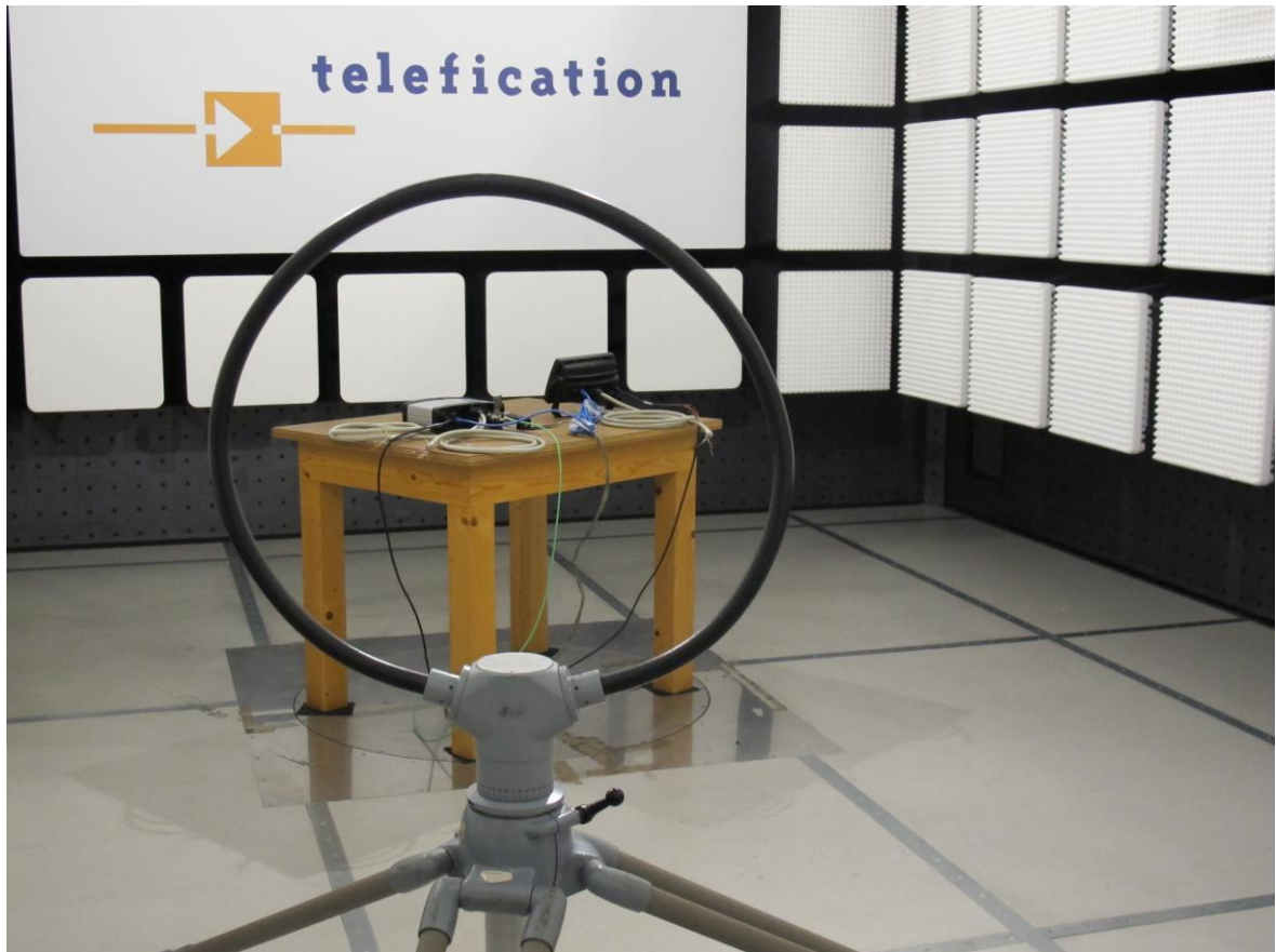
Photograph 6: radiated emissions test set up (0.15 – 30 MHz)
