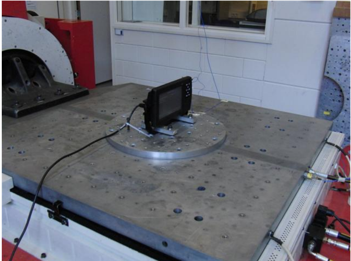
Photograph 10: Vibration test setup with R5 CDU in gimbal mounting frame (1 st horizontal direction)
