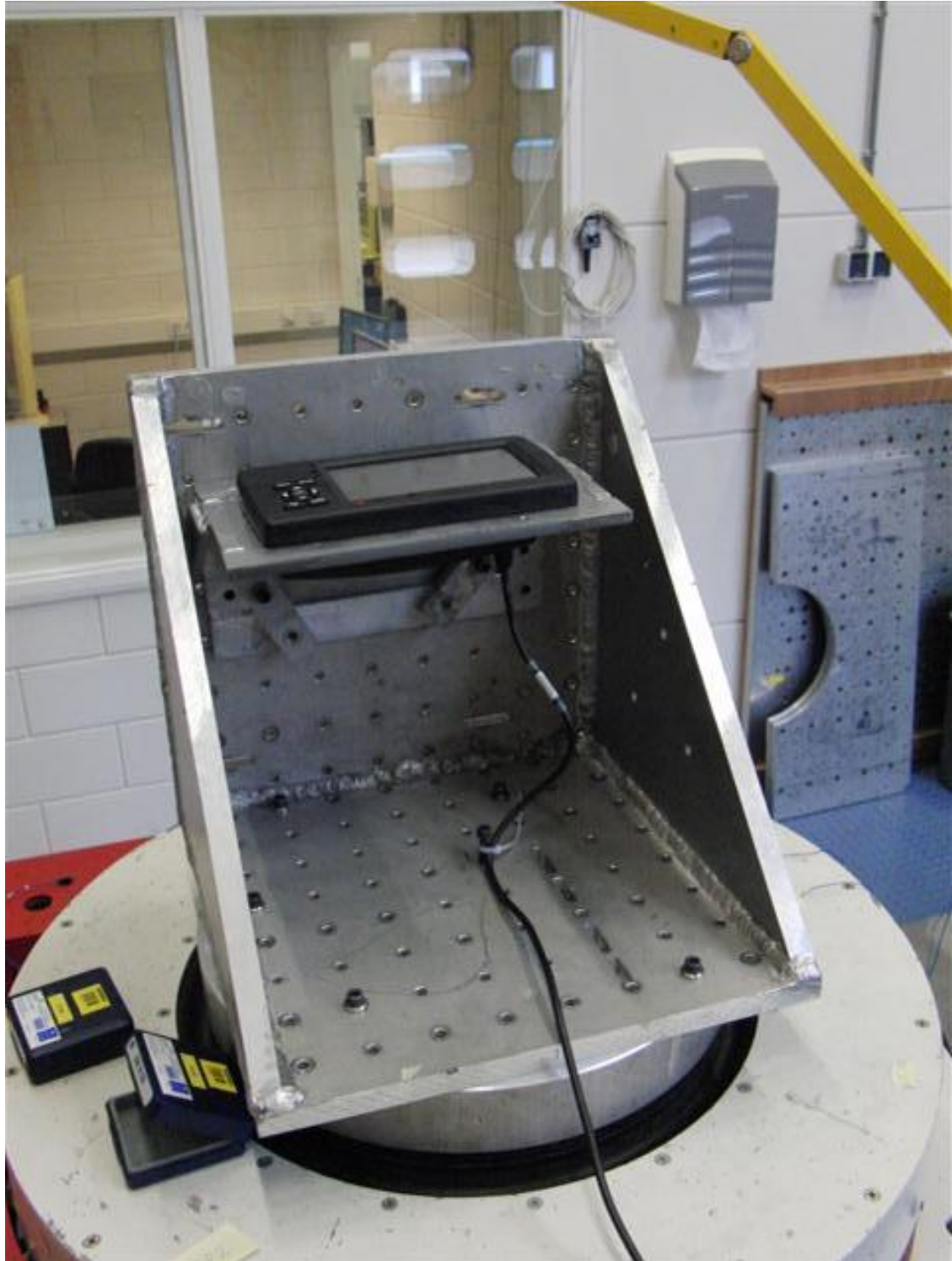
Photograph 15: Vibration test setup with R5 CDU in panel mounting frame (2 nd horizontal direction)
