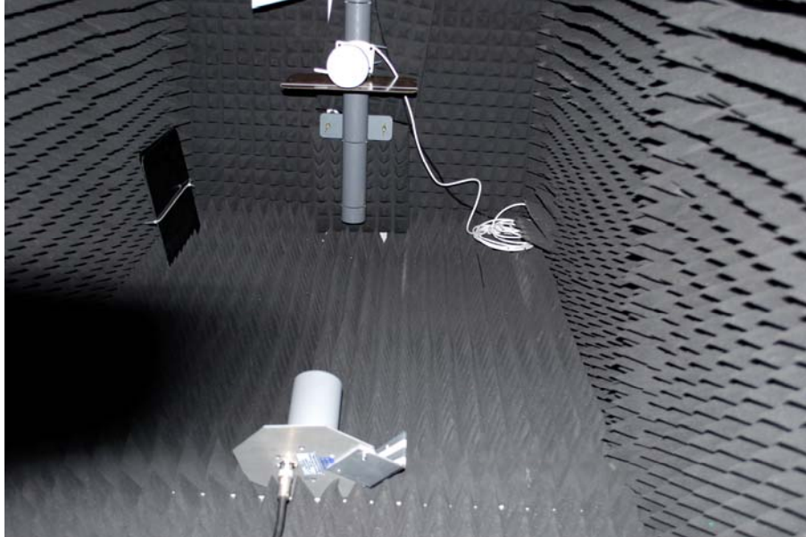
L-Band interference test – GPS Antenna Unit 1
