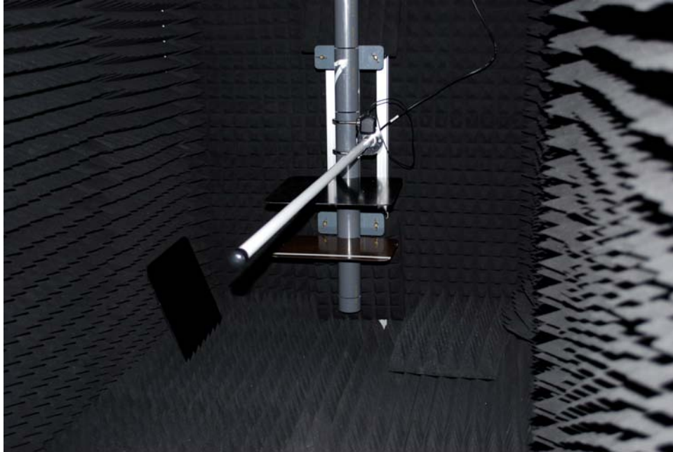
L-Band interference test – GPS Antenna Unit 3
