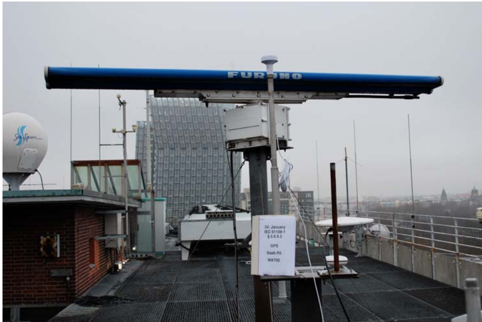
S-Band interference test – GPS Antenna Unit 1
