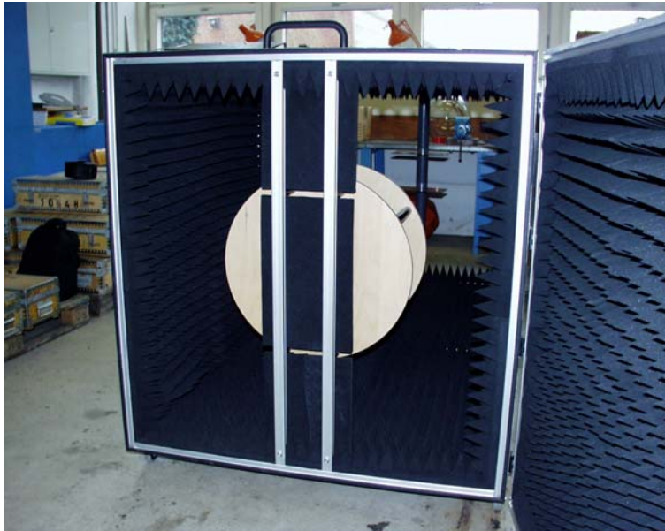
GPS test box, interior view
