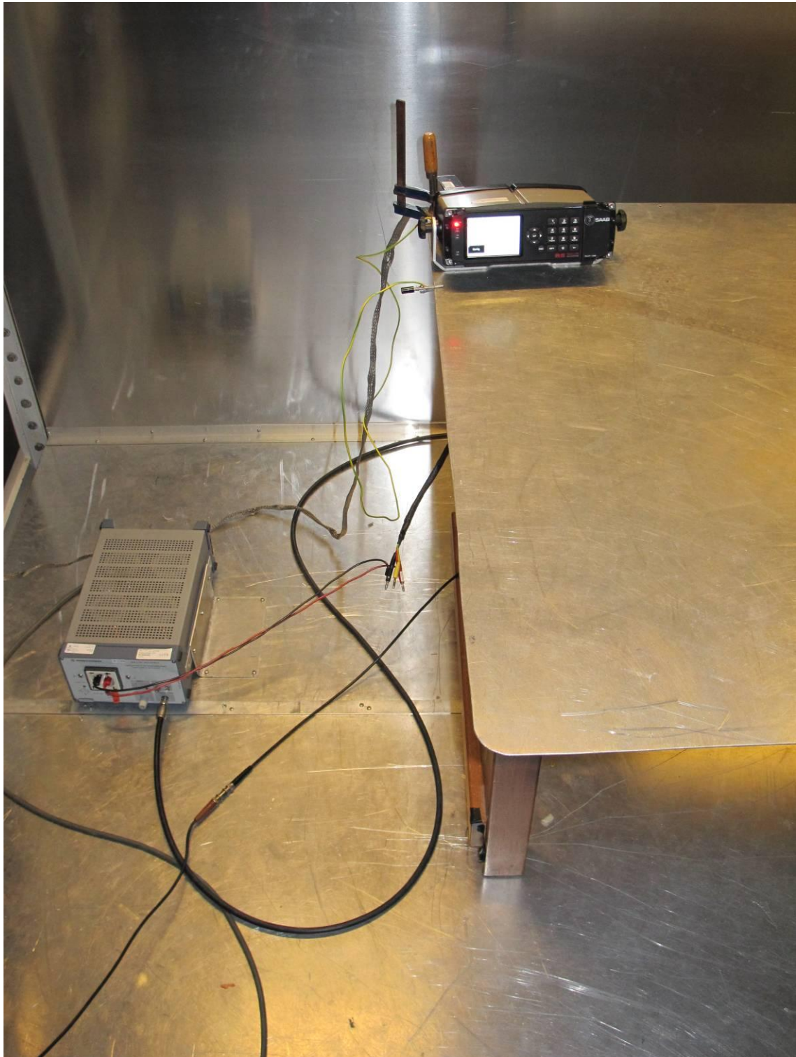
Photograph 3: Test setup conducted emissions (0.01 - 30 MHz)
