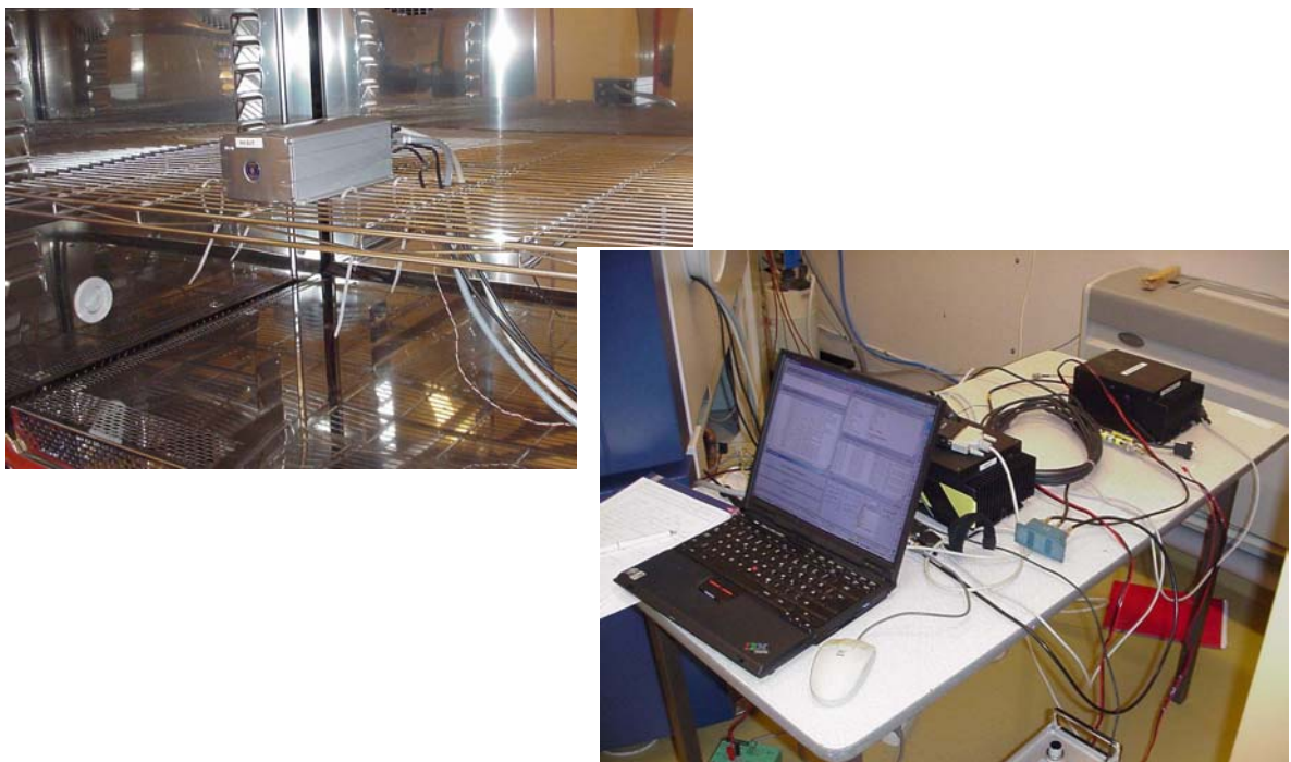
Figure 3 Test set up for “channel switching test” during climatic stress.
