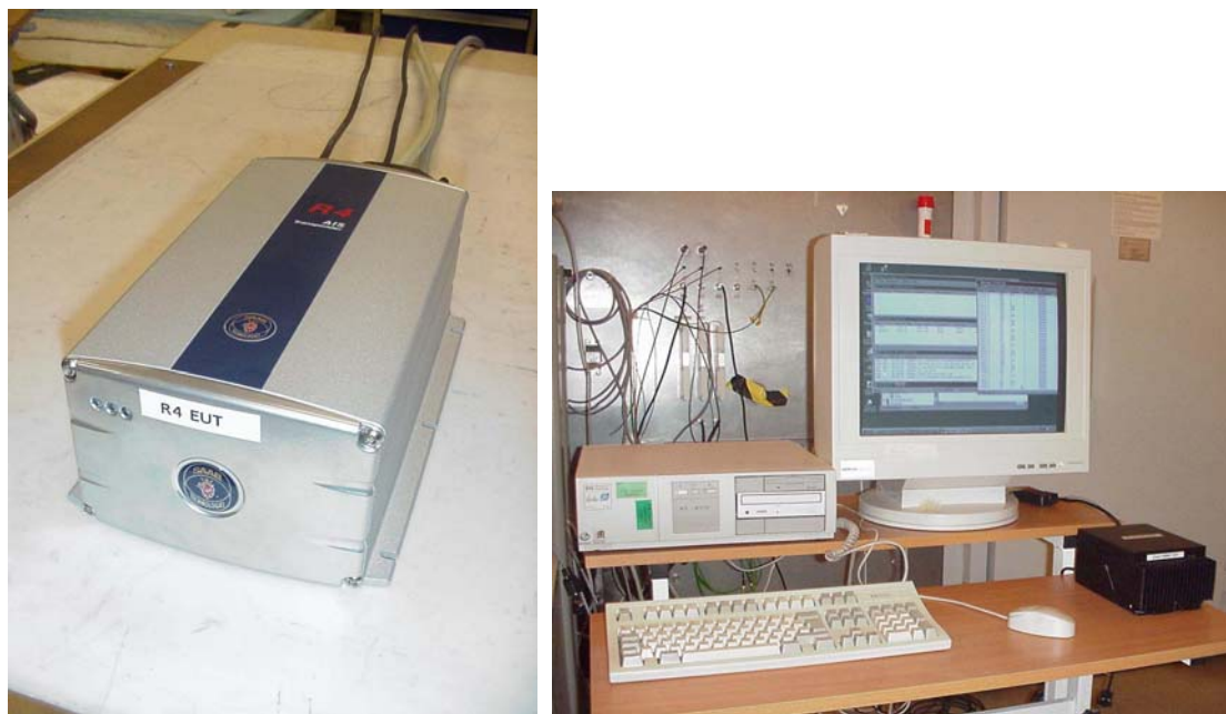
Photo 1 Left; EUT. Right; Auxiliary equipment (R3 transponder &amp; PC)
