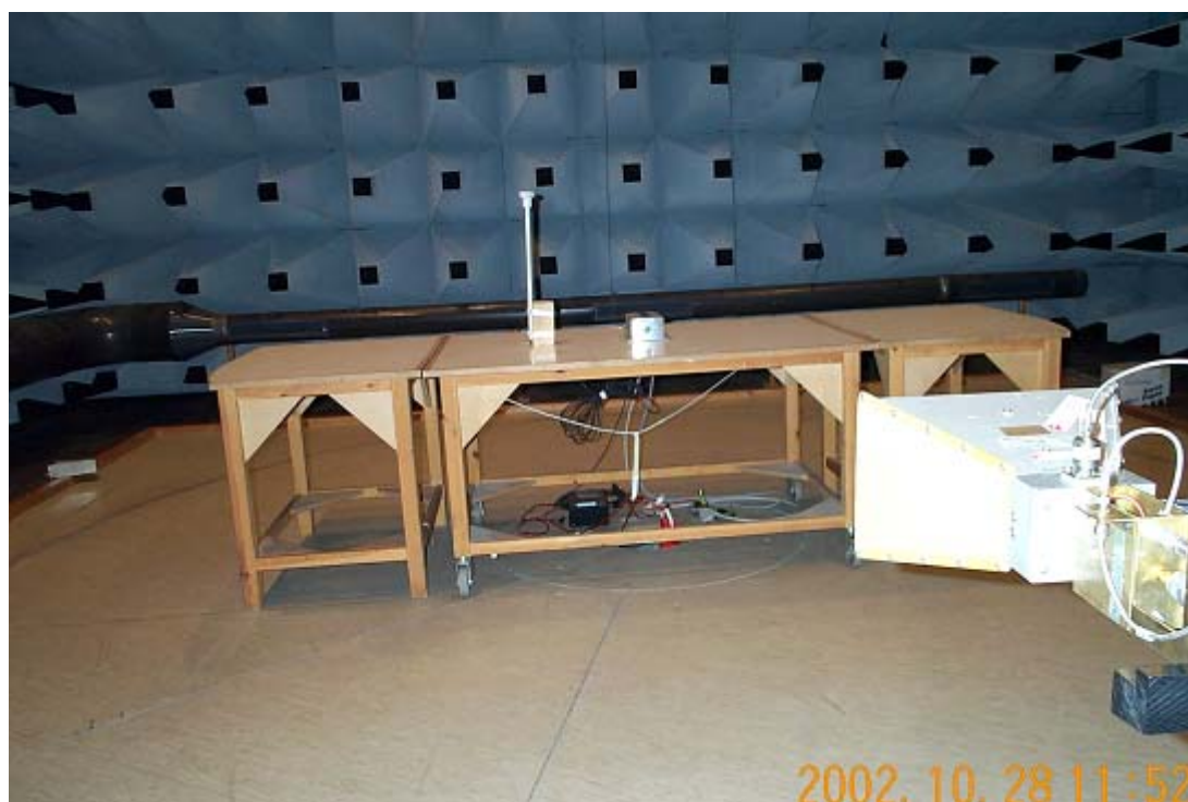
Photo 5 Test set up for radiated RF emission test. 1000 MHz - 2000 MHz.
