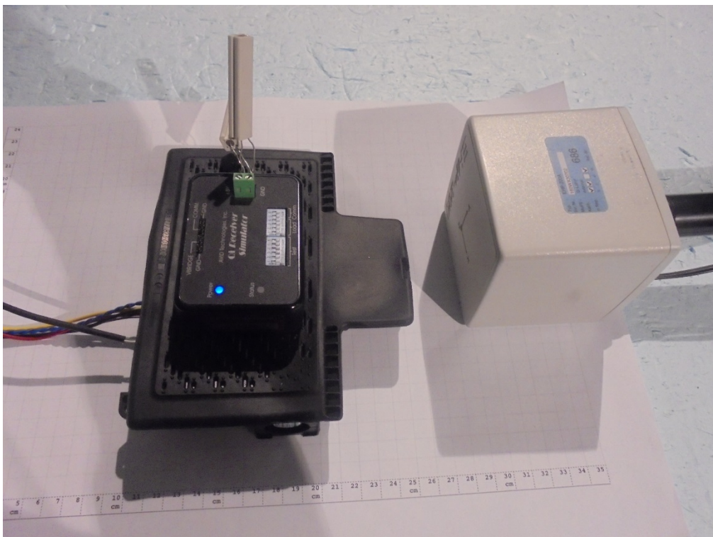
Photograph 10: Measurements in the anechoic chamber, 10cm distance between measurement probe and EUT, Position 4
