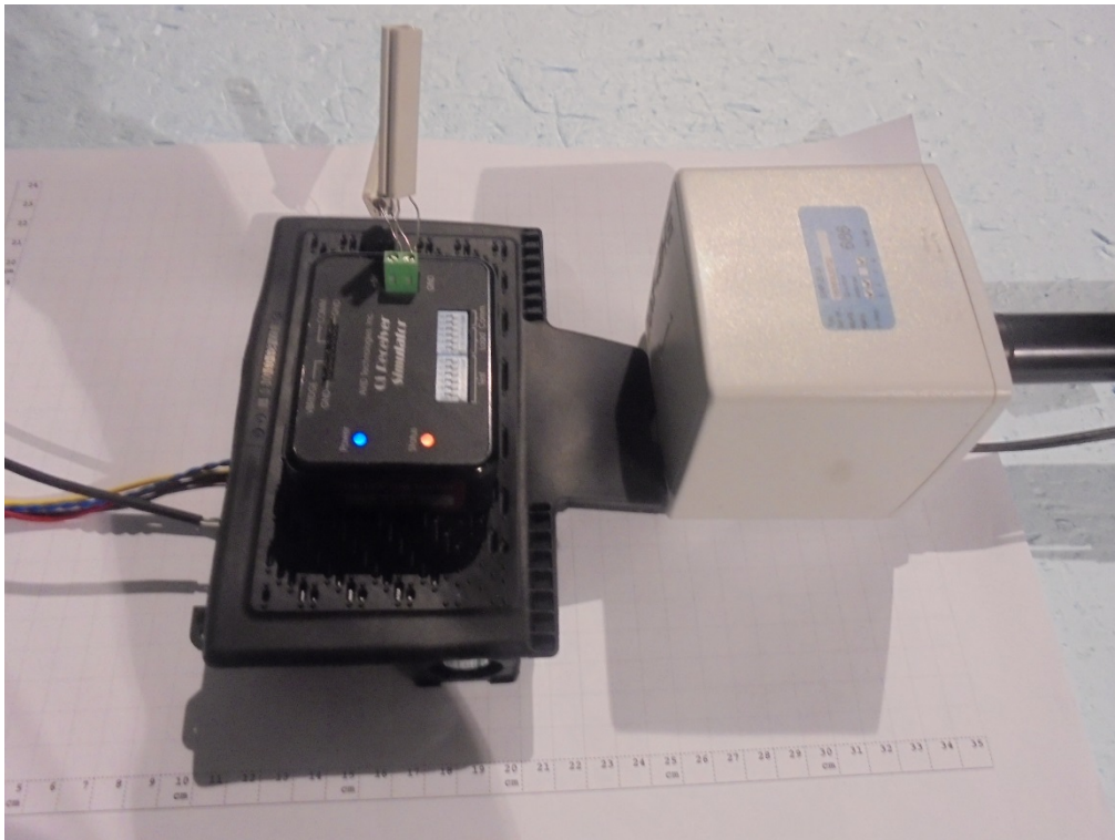
Photograph 9: Measurements in the anechoic chamber, 5cm distance between measurement probe and EUT, Position 4
