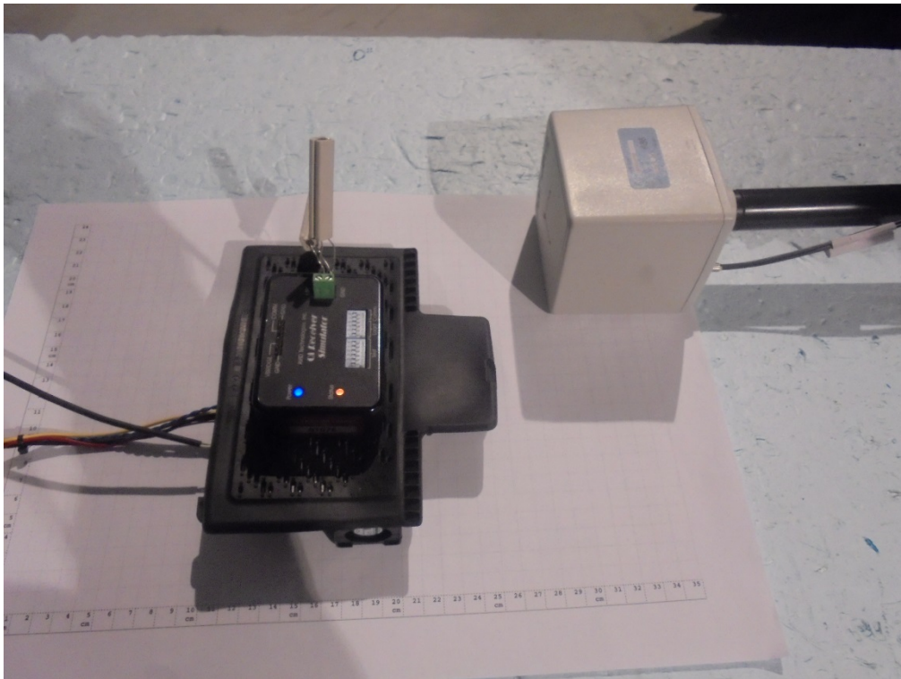
Photograph 15: Measurements in the anechoic chamber, 10cm distance between measurement probe and EUT, Position 6
