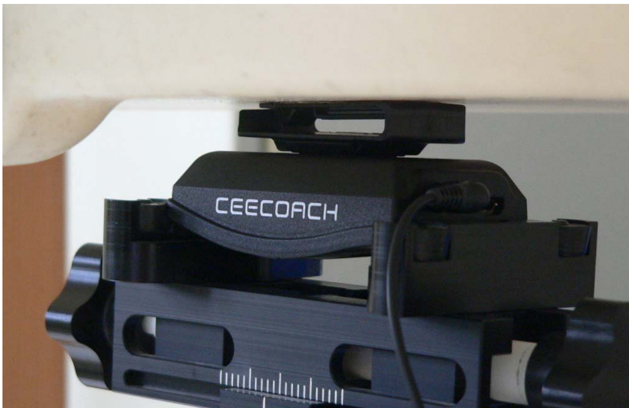
Fig. 11: Body worn configuration, headset and belt clip attached, back side toward the phantom, gap = 0 mm.
