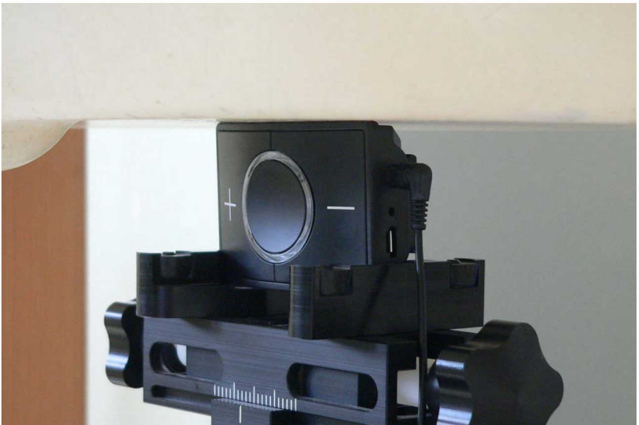
Fig. 13: Body worn configuration, headset and belt clip attached, top side toward the phantom, gap = 0 mm.
