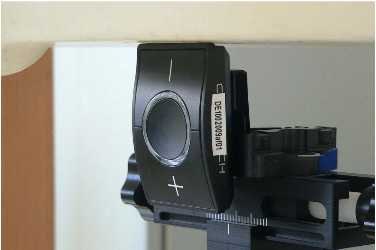
Fig. 15: Body worn configuration, belt clip attached, headset detached, right side toward the phantom, gap = 0 mm.
