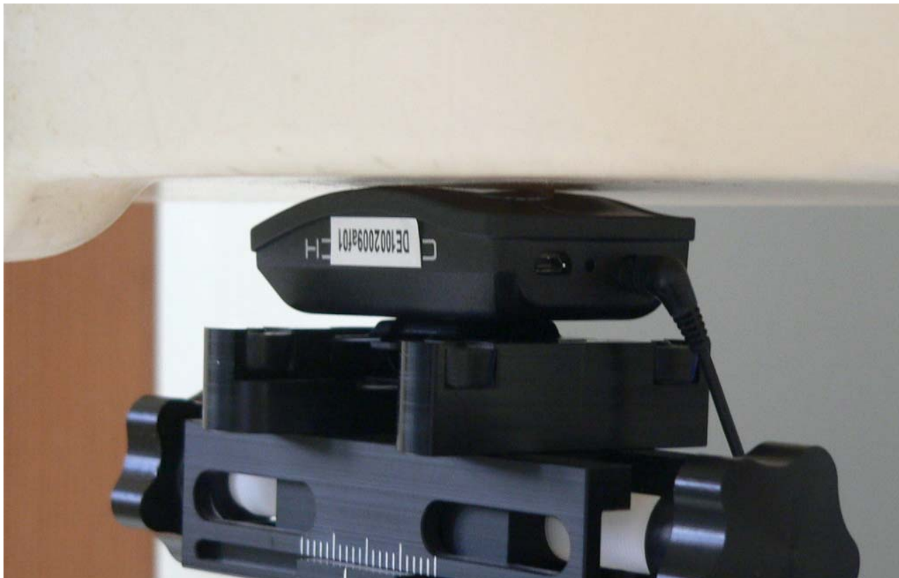
Fig. 10: Body worn configuration, headset and belt clip attached, front side toward the phantom, gap = 0 mm.
