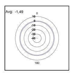
The "0 dBi" level is the level received by the reference antenna (lambda/4) placed on the roof in the same position of tyhe AUT
