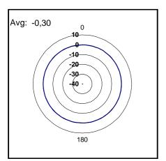
The "0 dBi" level is the level received by the reference antenna (lambda/4) placed on the roof in the same position of tyhe AUT
