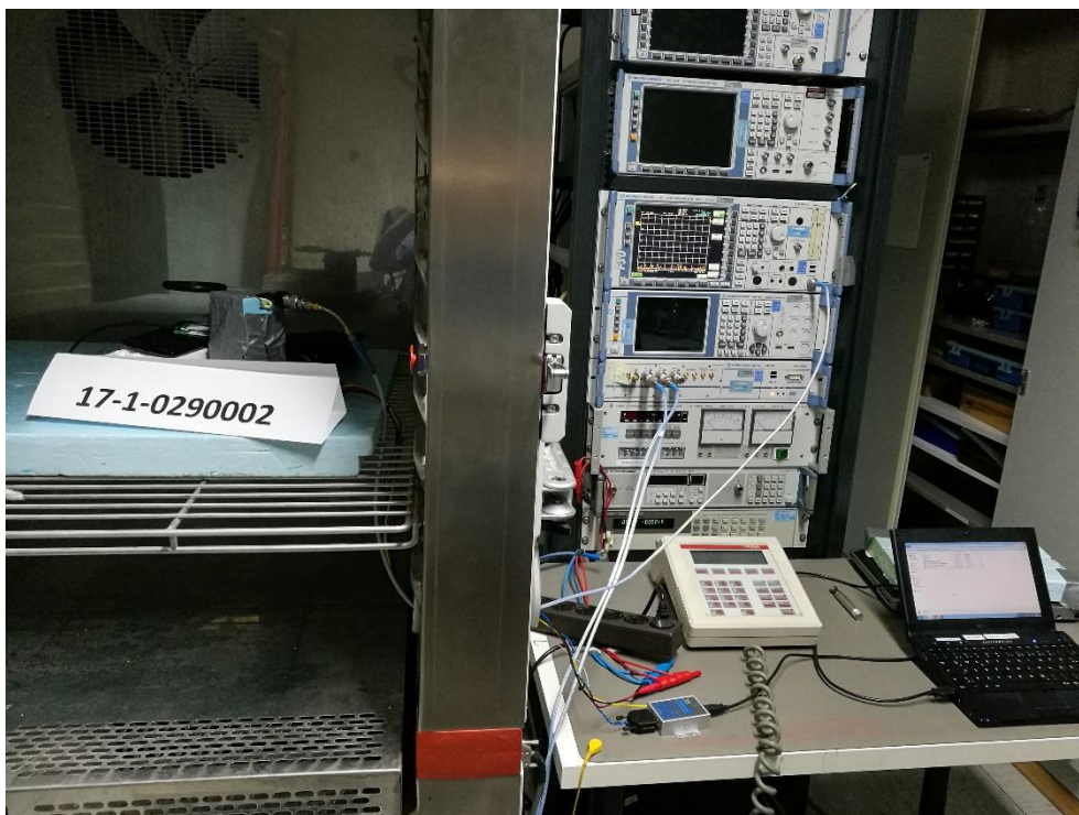
Photograph 2: EUT inside Temperature Chamber- Overall View
