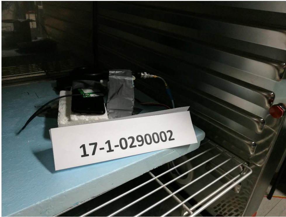
Photograph 1: EUT inside Temperature Chamber- Close View
