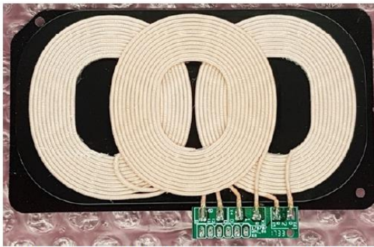
Charging coil module with ferrite plate, top and bottom view.
