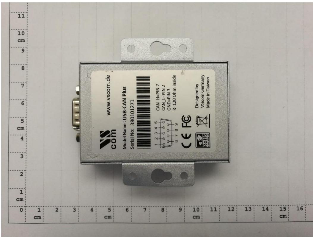
Diagram 6: AE 1 (VScom USB-CAN Adapter) back side
