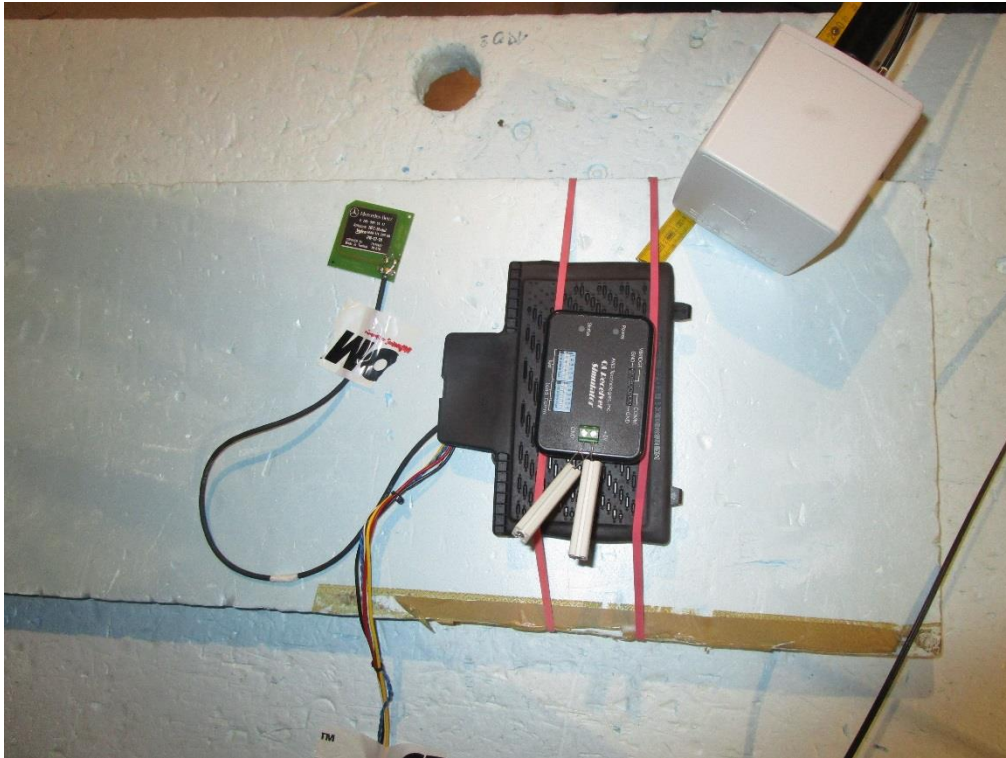
Photograph 5: Measurements in the anechoic chamber, 5cm distance between measurement probe and EUT, Position 3
