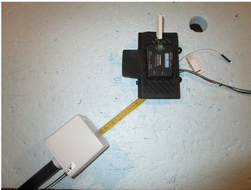
Photograph 2: Measurements in the anechoic chamber, 15cm distance between measurement probe and EUT, Position 1
