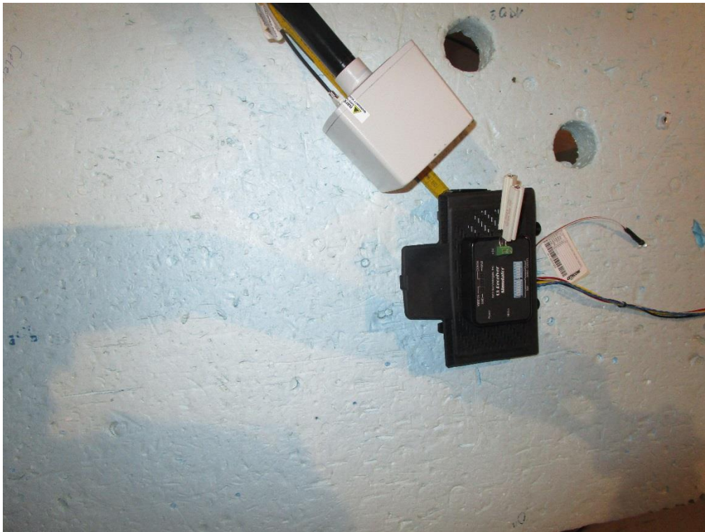
Photograph 3 Measurements in the anechoic chamber, 5 cm distance between measurement probe and EUT, Position 2
