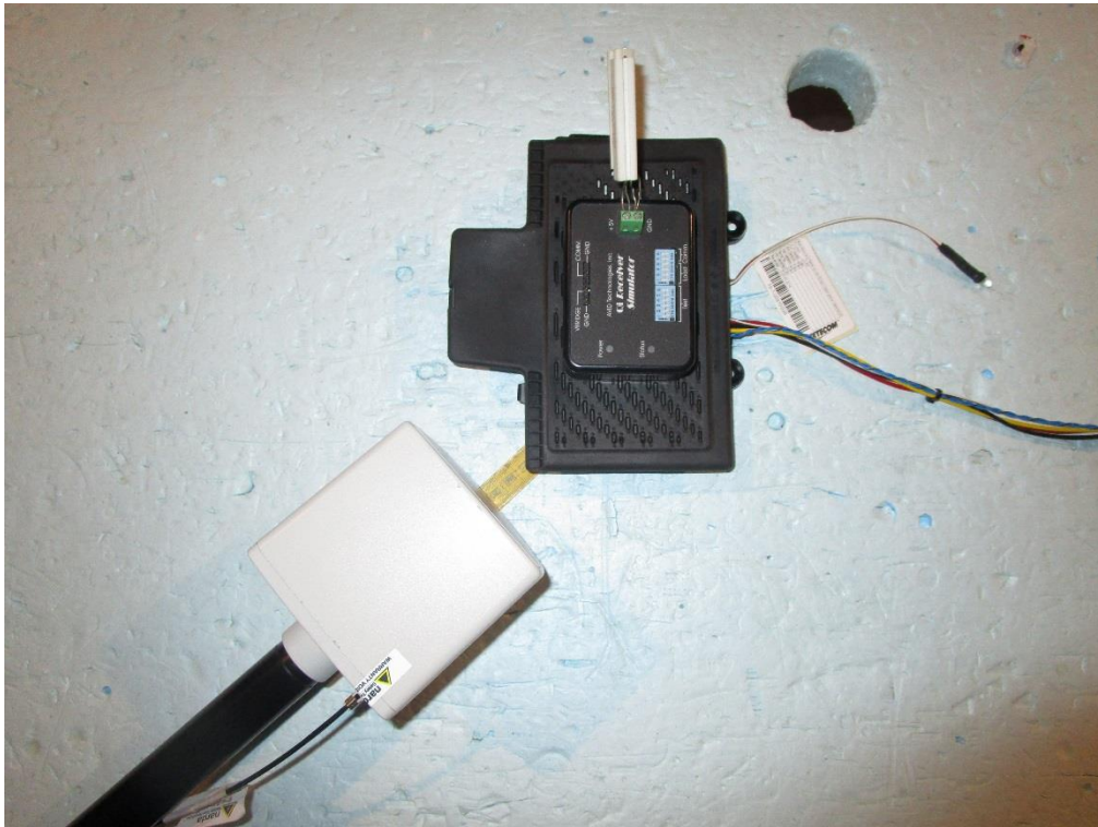
Photograph 1: Measurements in the anechoic chamber, 5 cm distance between measurement probe and EUT, Position 1
