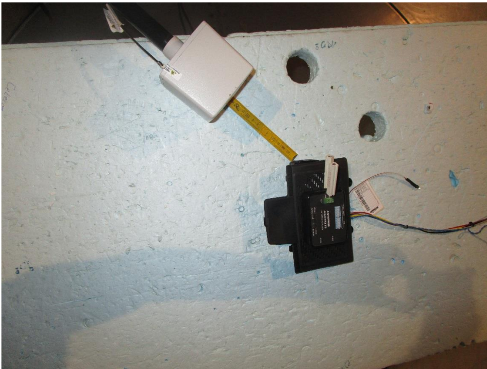
Photograph 4: Measurements in the anechoic chamber, 15cm distance between measurement probe and EUT, Position 2
