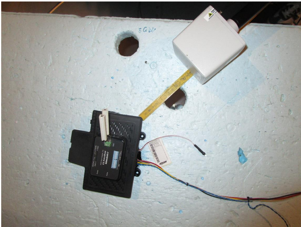
Photograph 6: Measurements in the anechoic chamber, 15cm distance between measurement probe and EUT, Position 3
