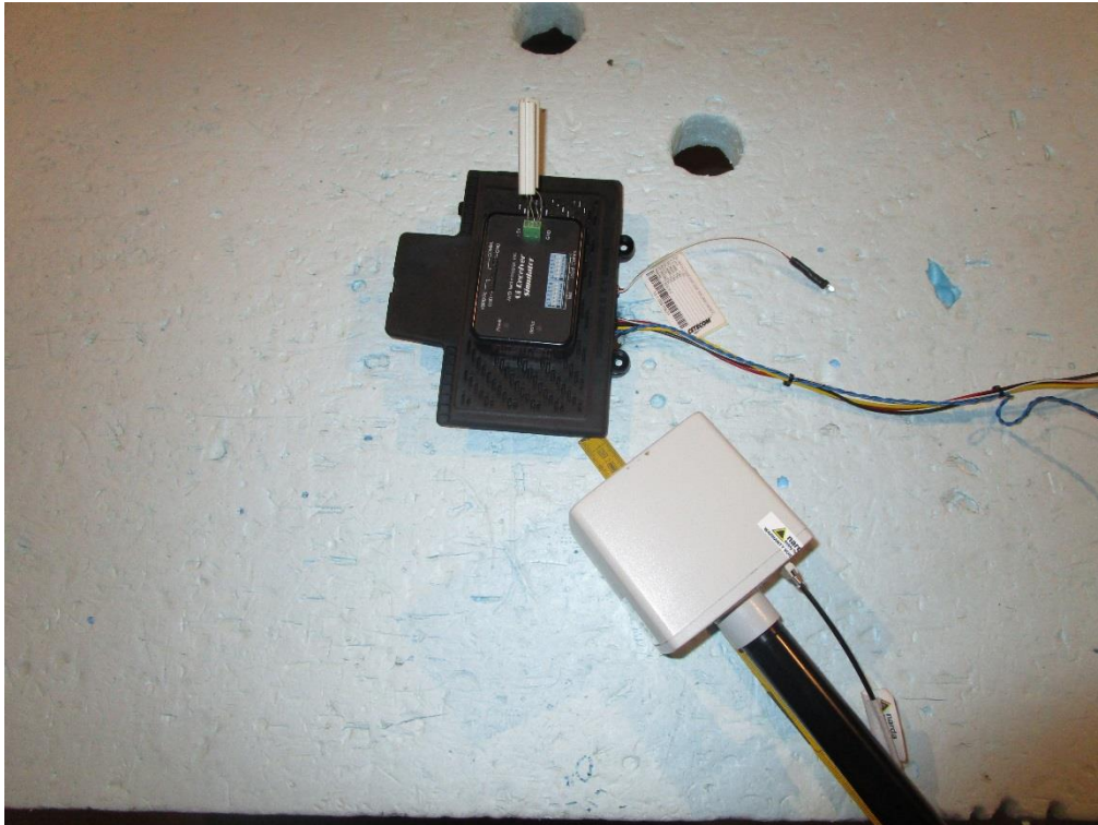
Photograph 7: Measurements in the anechoic chamber, 5cm distance between measurement probe and EUT, Position 4
