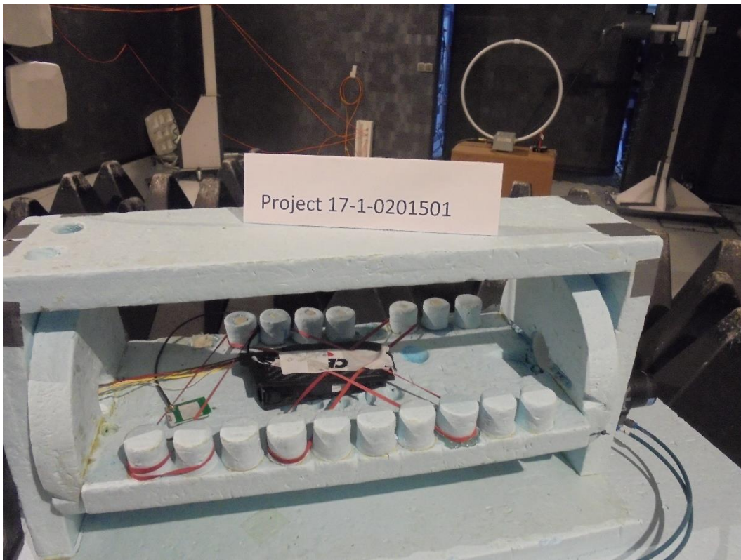
Photograph 4: Close View- 9 kHz-30 MHz- EUT laying – (Remark 1: This project number is also valid for this project. Remark 2: This test setup photograph is also valid for the test report CETECOM_TR17_1_0290002T09b.)
