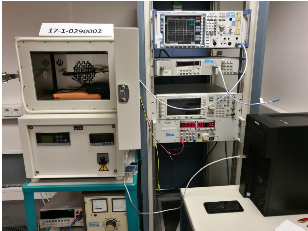
Photograph 1: EUT inside climate chamber- Overall View
