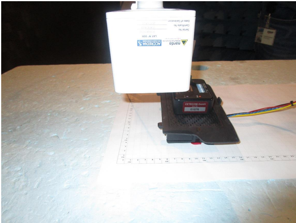
Photograph 3 Measurements in the anechoic chamber, 10cm distance between measurement probe and EUT, Position 1
