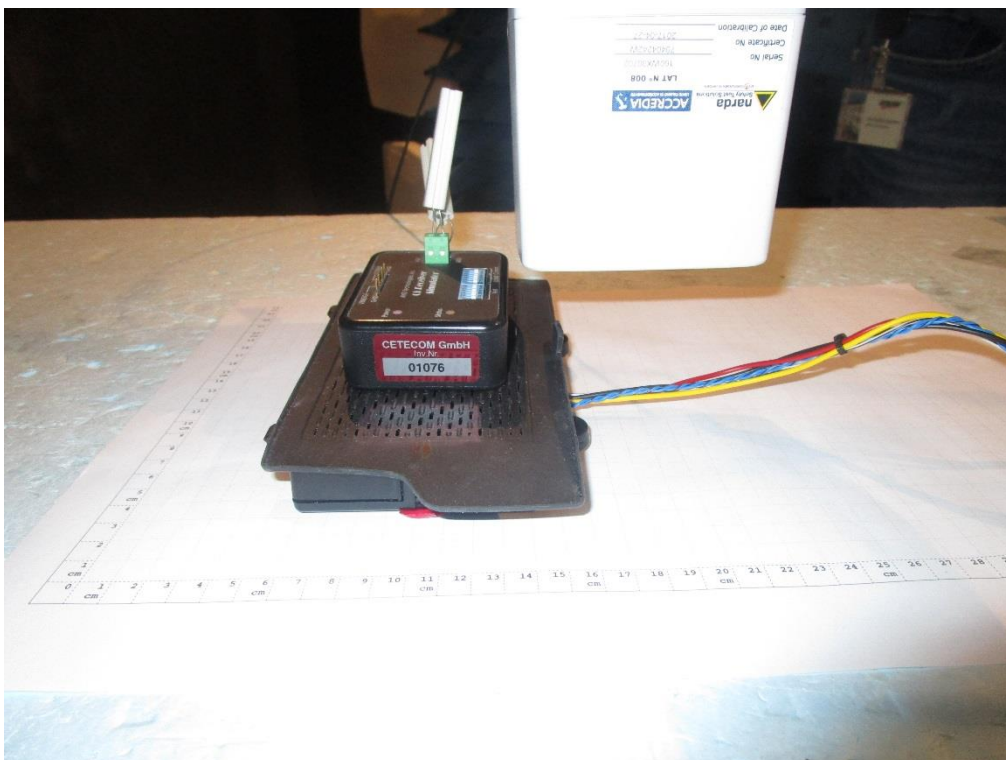
Photograph 12: Measurements in the anechoic chamber, 5cm distance between measurement probe and EUT, Position 4
