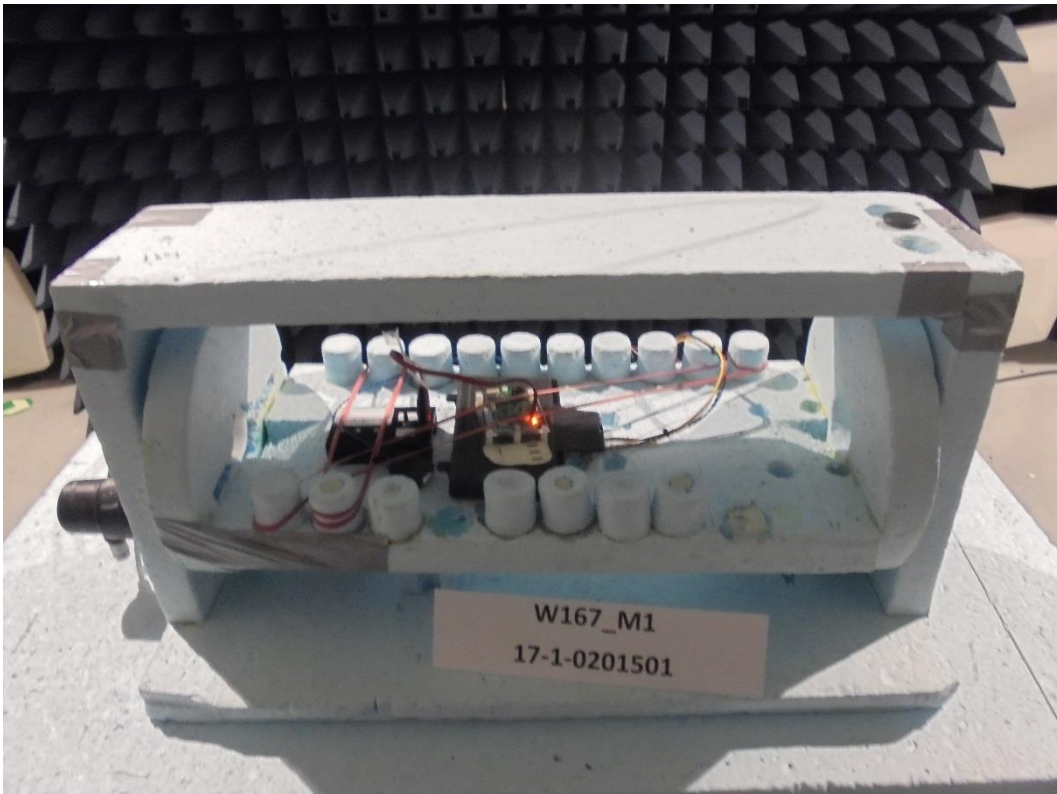
Photograph 4: Close View -9 kHz-30 MHz- EUT Laying - Front Side
