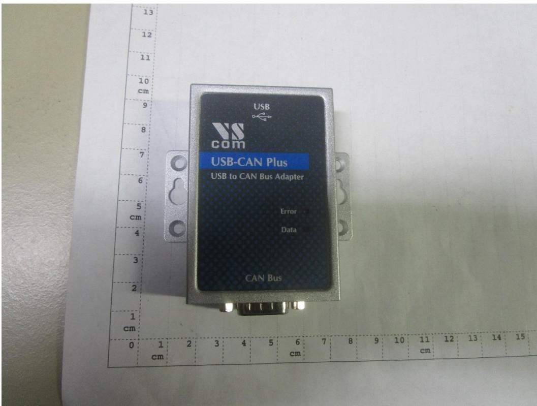
Photograph 6: AE 2- USB CAN Adapter
