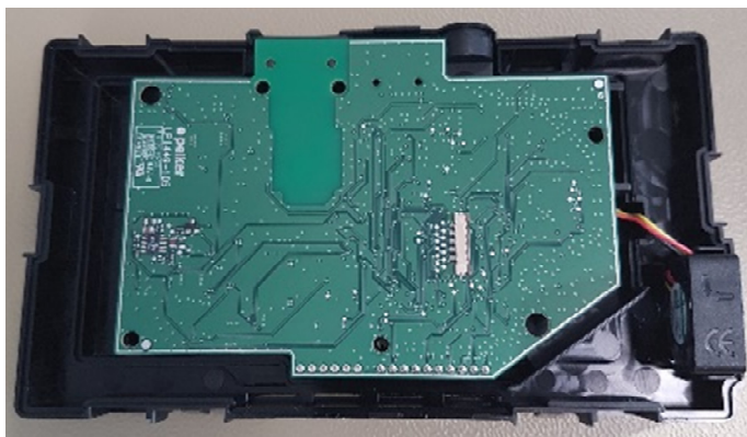
After removing Bottom-Housing, WMI2-W167 M1 looks like this. You see Main-Board with JTAG-Connector and Fan.
