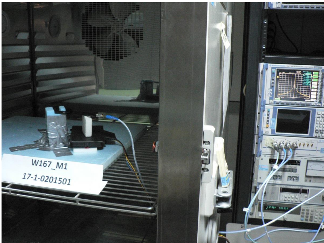
Photograph 2: EUT inside Temperature Chamber- Overall View
