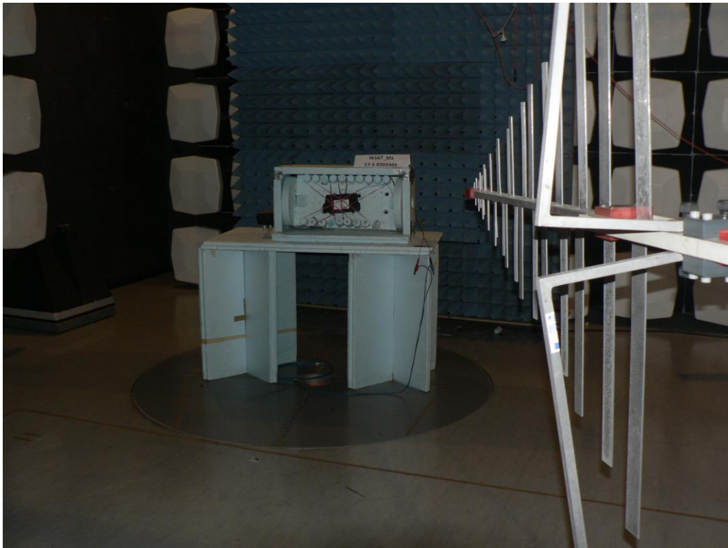
Photograph 5: Overall View- 30 MHz-1 GHz- EUT Laying - Front Side
