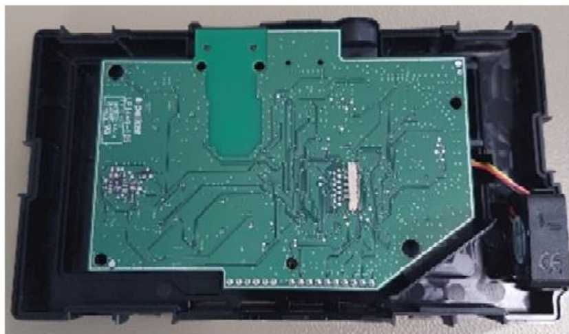
Main-Board with JTAG-Connector and Fan
